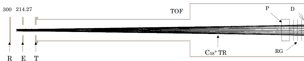
Fig. 1 Schematic 2D view of the imaging lens setup in combination with potential switch and kinetic energy analyzer. Trajectories of C_{58}^+ fragment ions having initial KE of 0.1 eV are drawn. R: Repeller; E: Extractor; T: Tube Electrode (grounded); TOF: TOF Tube; P: Potential switch; RG: Retarding grid; D: Detector.
