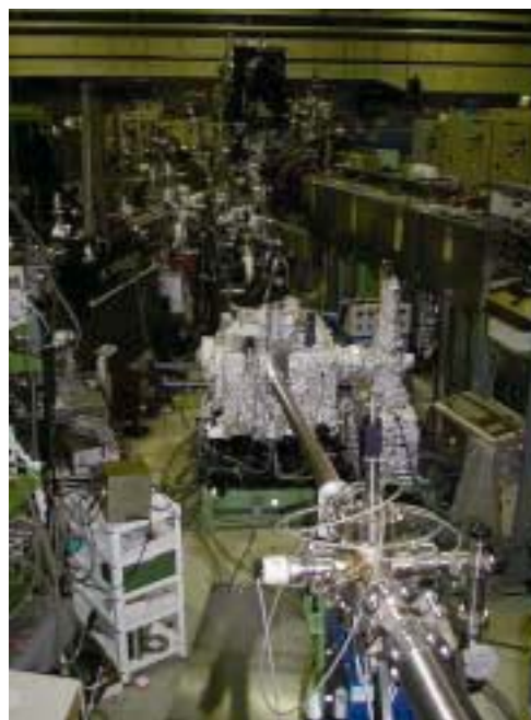
Fig. 1 18-m spherical grating monochromator installed at the Beamline 2B.
