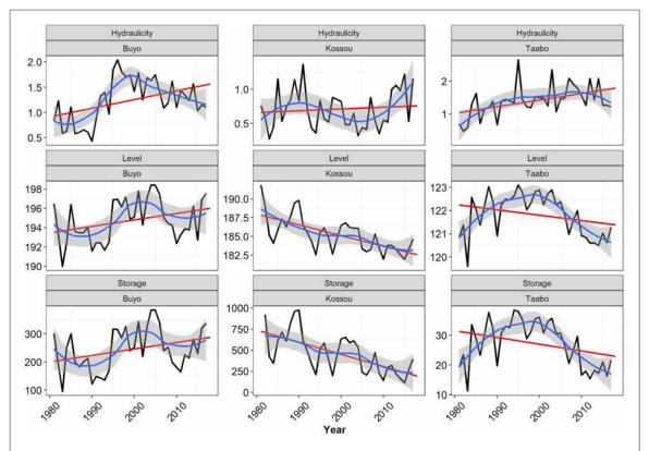
**Figure 6.** Interannual variability of hydraulicity indices (1st row), water level (2nd row), and water storage (3rd row) at Buyo (1st column), Kossou (2nd column), and Taabo (3rd column) hydropower plants over 1981–2017 period. The red line is the linear regression line, the blue line represents the smoothing curve while the grey area (span) gives the proportion of points in the plot which influence the smooth at each value.
