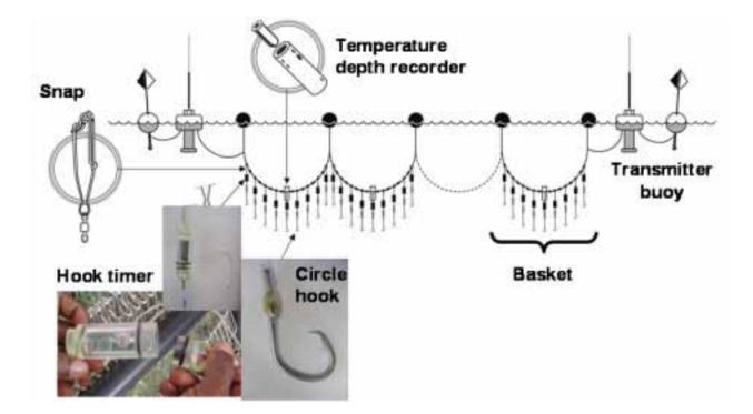
Figure 6 - The instrumented longline deployed during the SWIOFP ILL training cruise
