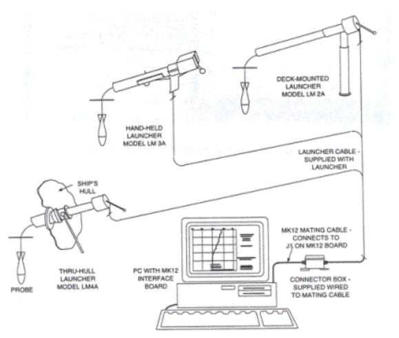
Figure 3 – Design of the Sippican's XBT system used to carry out temperature – depth profiles (Source : <u>http://www.sippican.com</u>).
