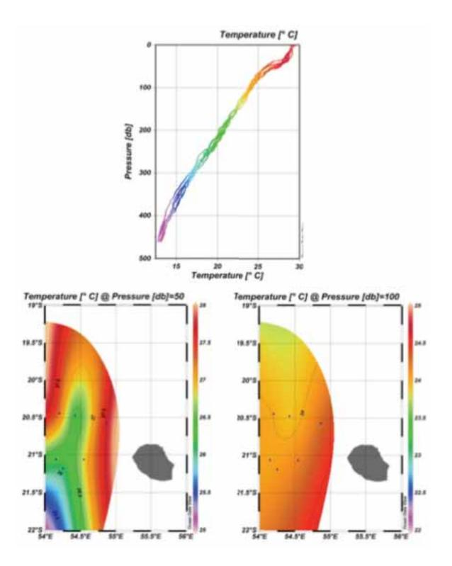
Figure 9 – Depth – temperature XBT profiles obtained during the ILL training cruise (top). Kriging map of the water temperature at 50 m depth (down left) and 300 m (down right) obtained from XBT profiles.
