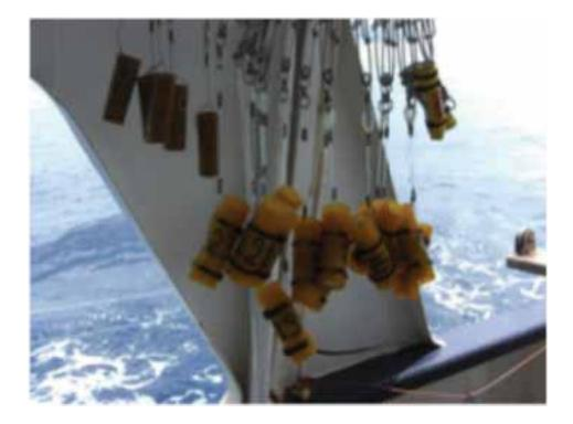
Figure 7 – TDRs ready to be deployed on the mainline
