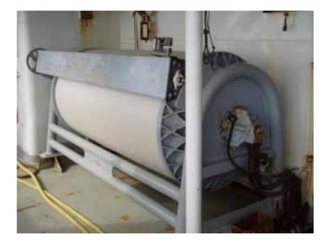
Figure 5 - The mainline spool by Lindgren Pitman  $^{\rm {\scriptscriptstyle TM}}$  installed on board the longliner
