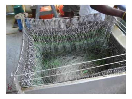
Figure 8 - Set of branchlines equipped with hook timers in its box.
