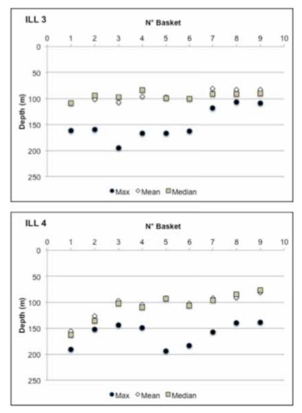
Figure 10 C, D – Maximum, mean and median of depth series recorded by TDRs on baskets of the instrumented longline fishing experiments 3 (ILL 3) and 4 (ILL4).
