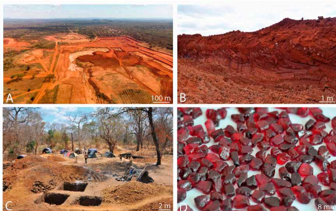
Figure 54. The placer deposits in the Montepuez mining district in Mozambique. (A) Aerial view of the Mugloto Pit operated by the Gemfields Group Ltd. The miners are using a back-filling technique (top) and using tree plantations for rehabilitation (bottom); (B) the ruby-rich gravel layer at Mugloto in the Montepuez mining district. The detritic levels contain sub-angular quartz and clay pebbles located between 4 and 10 m under the surface. Gemfields removes the overburden and uses an excavator to collect this gravel layer, that is then sent to the wash plant to extract rubies; (C) small scale miners near Nacaca village, an area reserved for locals outside the southeast border of the Gemfields concession, where a few thousand people have worked since 2012. At this location small rubies are found in gravels under to 2–5 m of overburden. The Nacaca stones are usually smaller and contain more inclusions than those from Mugloto and their iron content is similar to that of the material from Maninge Nice; (D) parcel of rough rubies from Mugloto Pit near Montepuez (about 0.5 g per stone) at a Gemfields rough ruby auction in Singapore. The rubies coming from a gravel layer range from bright to dark red (depending on their iron contents), and present some abrasion features. The area was discovered in early 2014 and probably more than 90% of Gemfields income since then has been extracted from this deposit. Photo: Vincent Pardieu © GIA.
