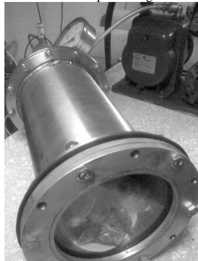
Figure 3. Stainless steel vessel covered with high resistant transparent polycarbonate flange/plate
