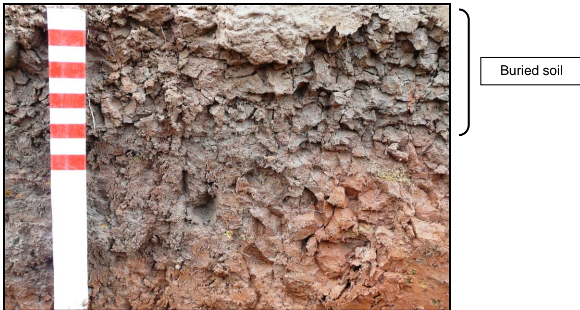
Plate 28: Buried soil developed in alluvium in trench 3. It marks a stabilisation and sealed with deposits which are more colluvial (hillwash) dominated.
