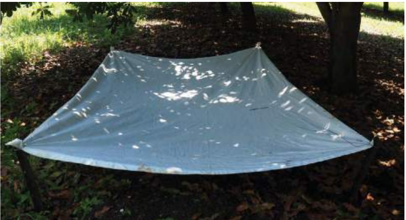
Figure 36. A drop sheet in place, under the canopy, with the corners raised.
