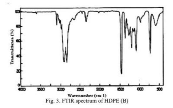
Figure A1.2, FT-IR spectra from three different types of high-density polyethylene (HDPE). Reproduced unedited from Charles, 2009. Original caption reads: "Spectroscopically pure sample of high-density polyethylene (HDPE) has been procured from Central Institute of Plastic Engineering and Technology (CIPET), Chennai, India."
