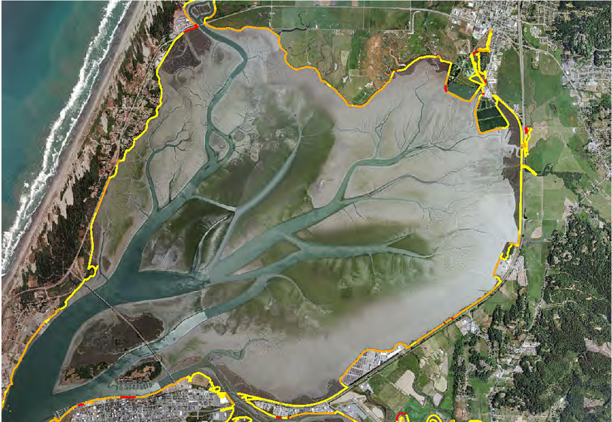
Figure 46. Distribution of shoreline cover types on Arcata Bay: vegetated (yellow), fortified (brown), and exposed (red).
