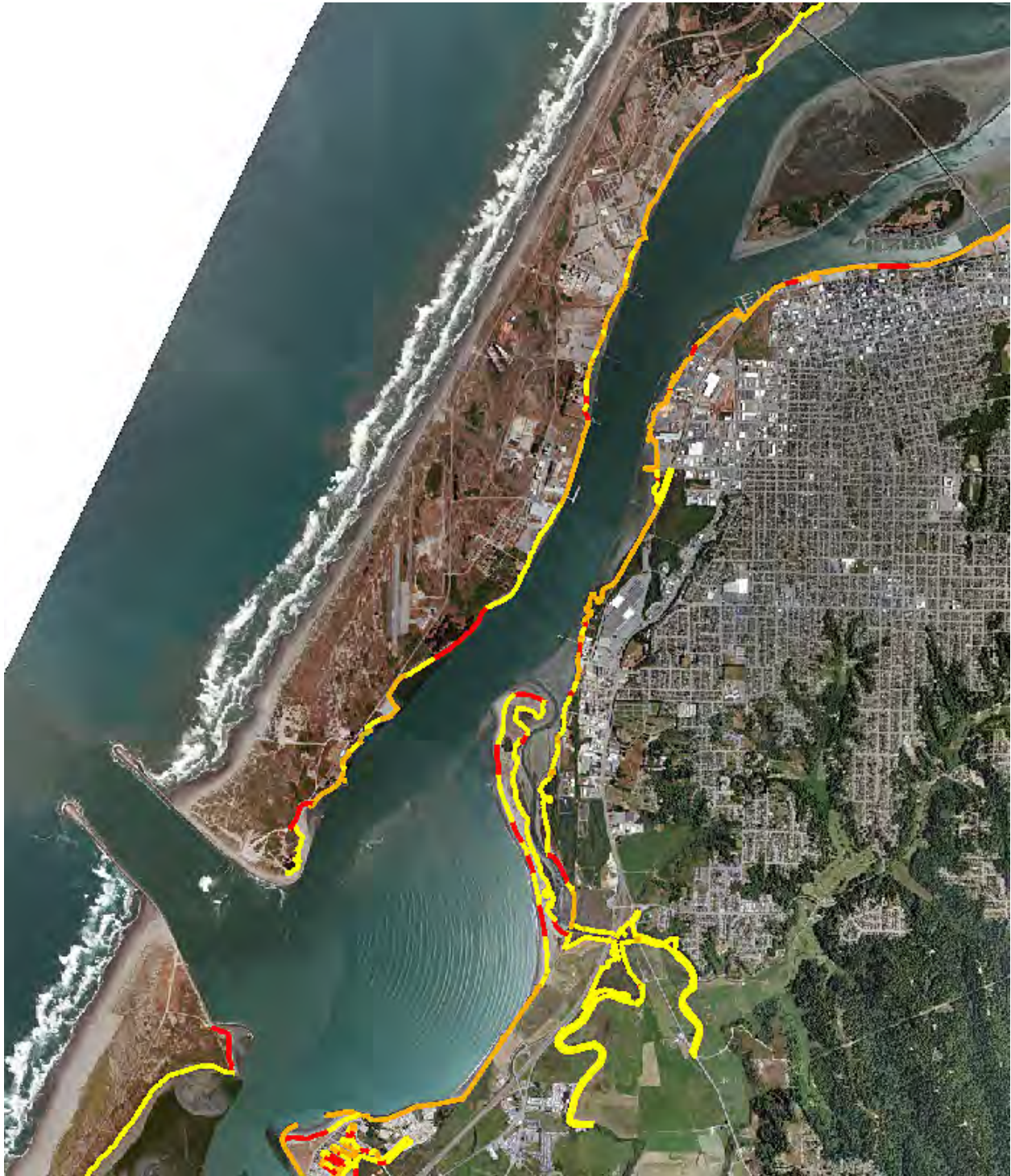
Figure 47. Distribution of shoreline cover types on Eureka Bay: vegetated (yellow), fortified (brown), and exposed (red).
