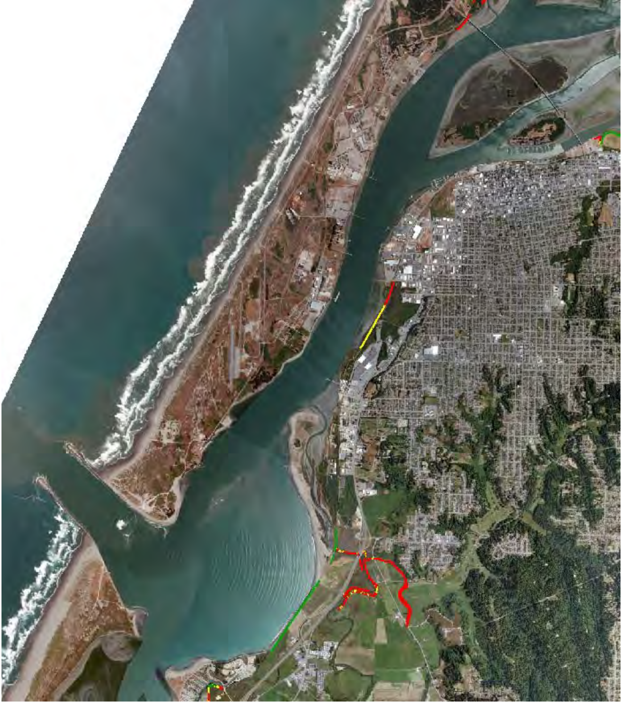
Figure 5. Diked and railroad shoreline vulnerability rating for Eureka Bay; red high, yellow moderate, and green low.
