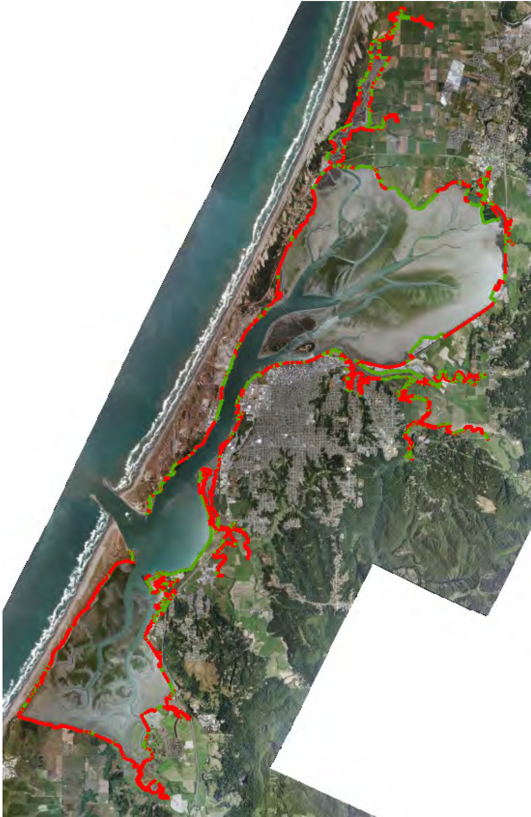
Figure 55. Humboldt Bay shoreline segments with elevations less than or equal to 10.74 feet (red) and segments that are greater than 10.74 feet in elevation (green).
