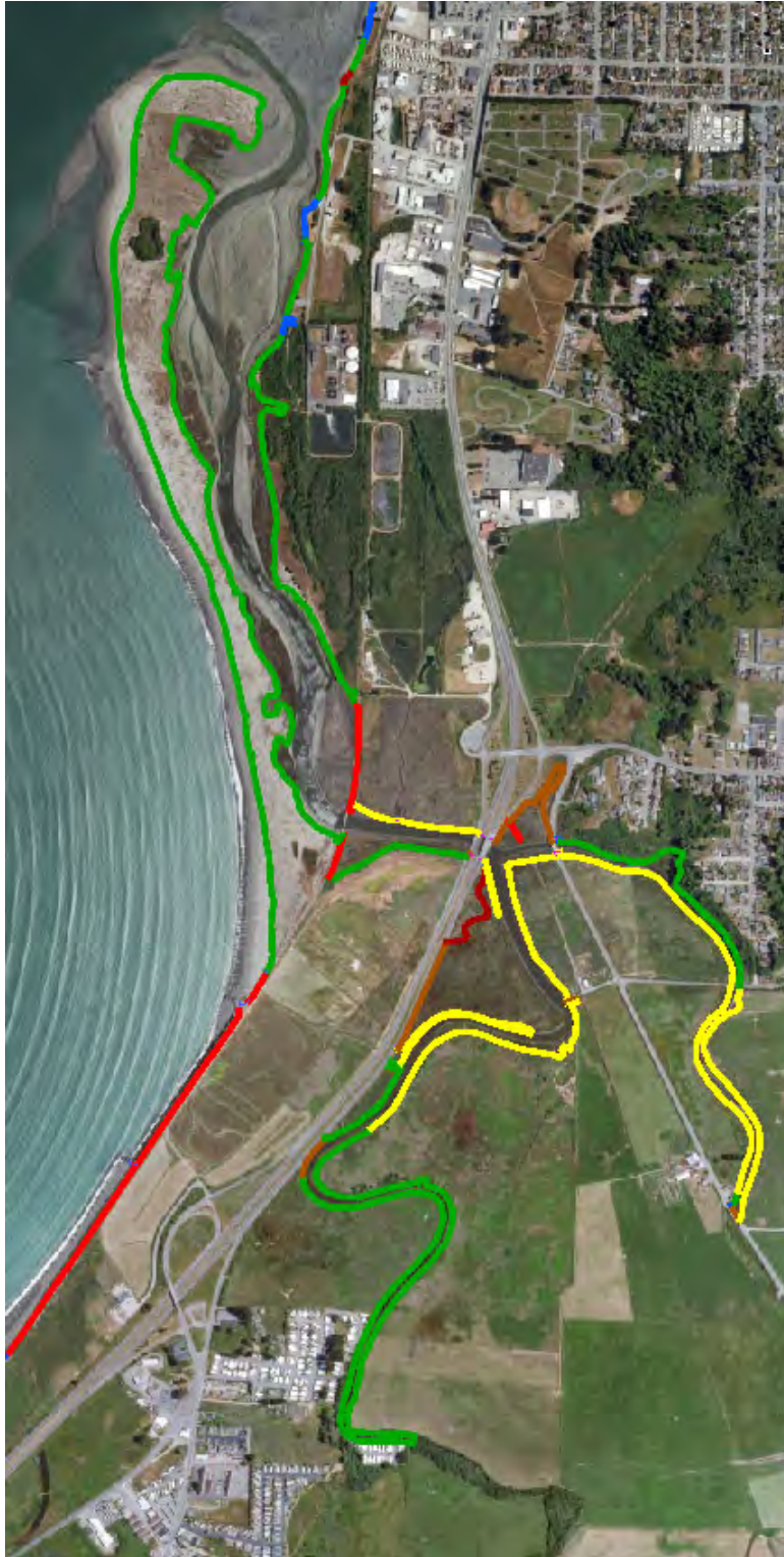
Figure 42. Distribution of shoreline structure types on Elk River Slough: dike (yellow), natural (green), railroad (red), fill (maroon), fortified (blue), and roadway (brown).
