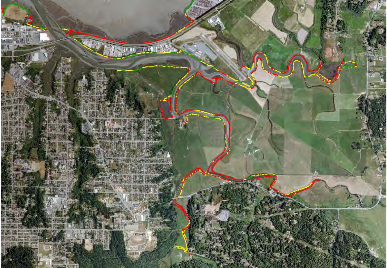
Figure 8. Diked and railroad shoreline vulnerability rating for Eureka Slough; red high, yellow moderate, and green low.
