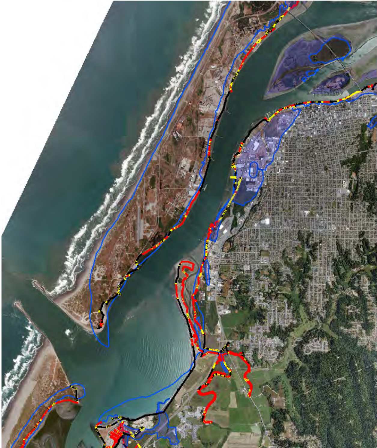
Figure 78. Eureka Bay, shoreline areas overtopped by 2 foot of sea level rise (red), and 3 feet (yellow), and the 1870 tidal inundation footprint (blue).
