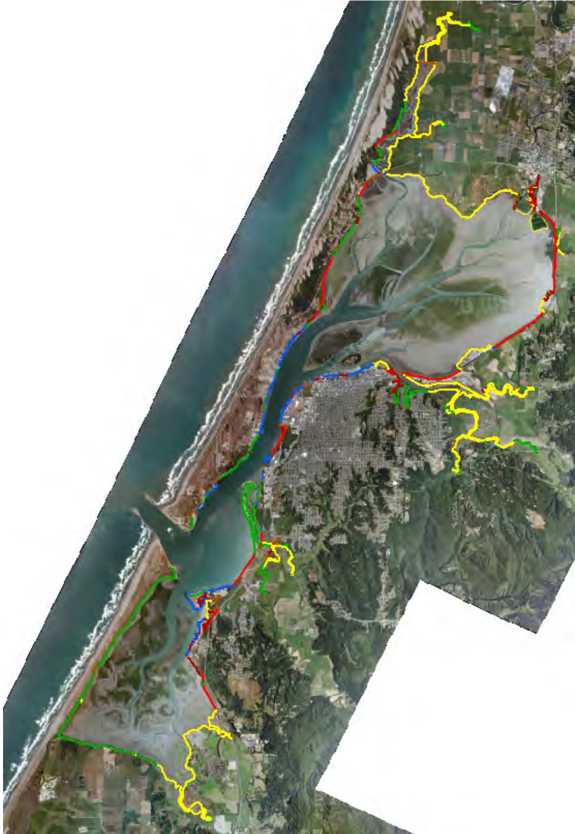
Figure 36. Distribution of shoreline structure types on Humboldt Bay: dike (yellow), natural (green), railroad (red), fill (maroon), fortified (blue), and roadway (brown).
