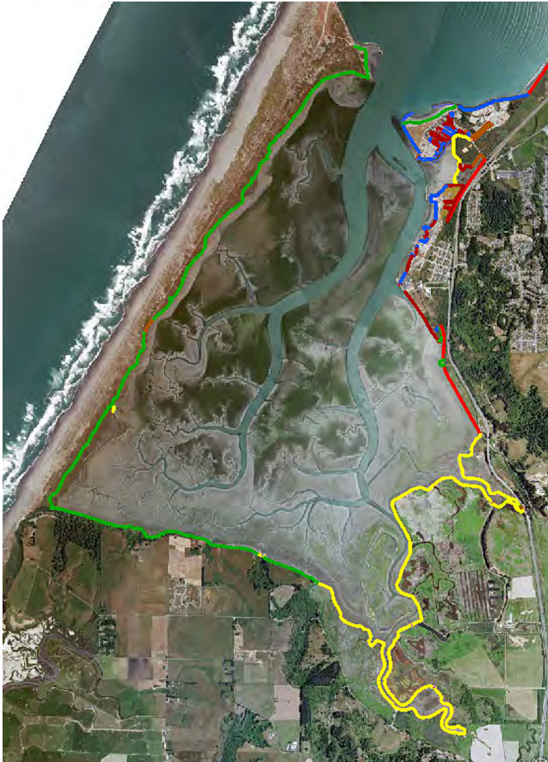
Figure 39. Distribution of shoreline structure types on South Bay: dike (yellow), natural (green), railroad (red), fill (maroon), fortified (blue), and roadway (brown).
