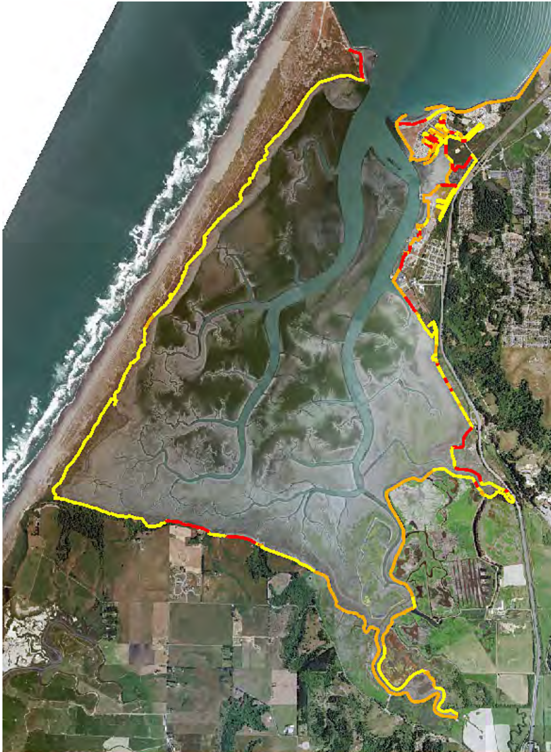
Figure 48. Distribution of shoreline cover types on South Bay: vegetated (yellow), fortified (brown), and exposed (red).
