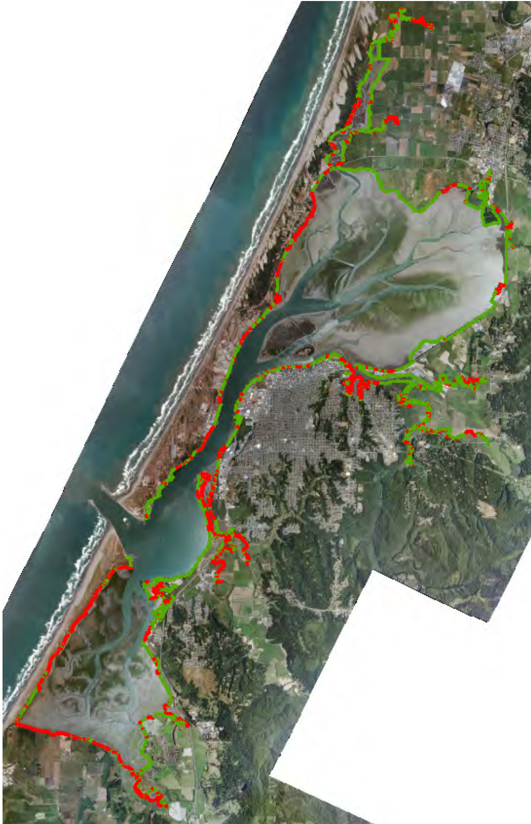
Figure 54. Humboldt Bay shoreline segments with elevations less than or equal to 9.74 feet (red) and segments that are greater than 9.74 feet in elevation (green).
