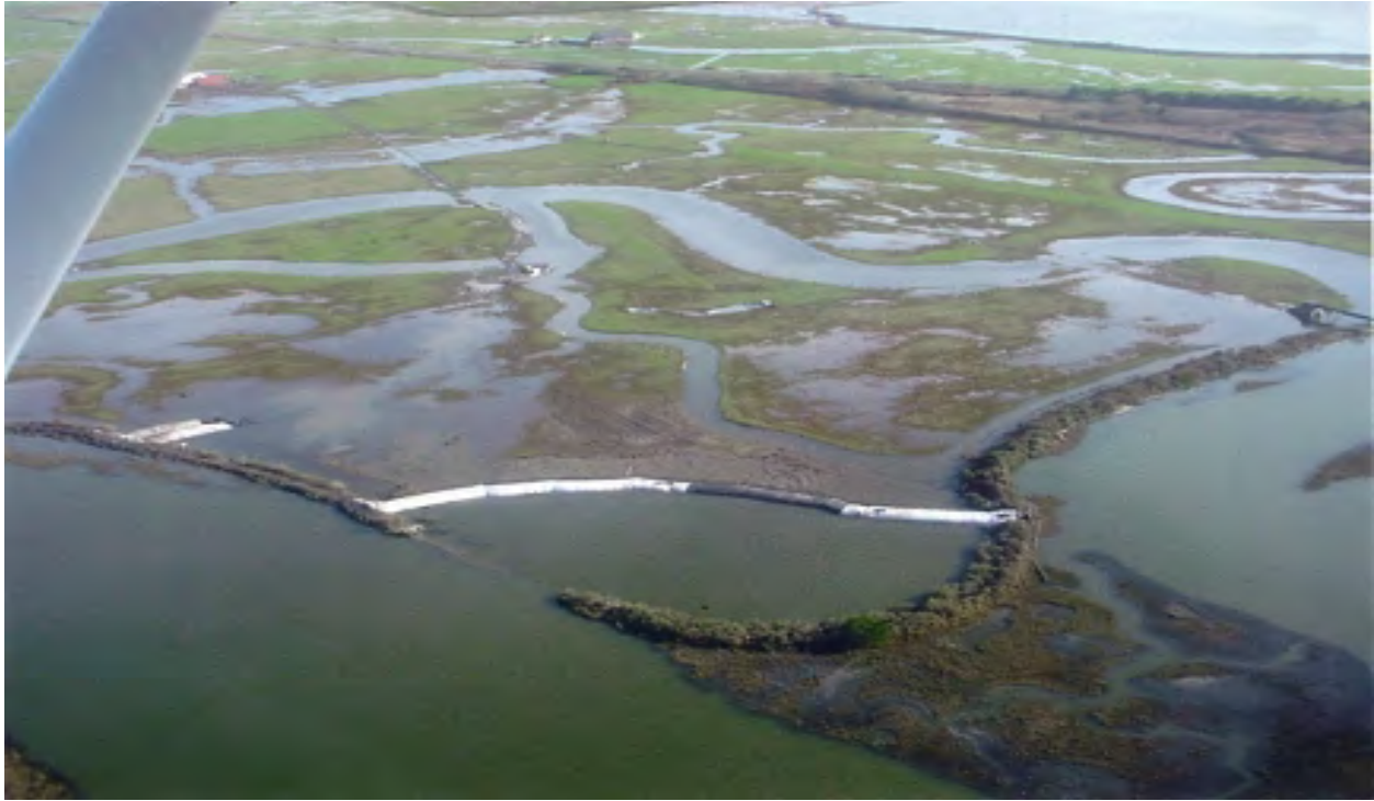
Figure 3, 2003 breach on Mad River Slough, 9.51 foot tide and storm surge (Times Standard, Andrew Bird, January 26, 2004).
