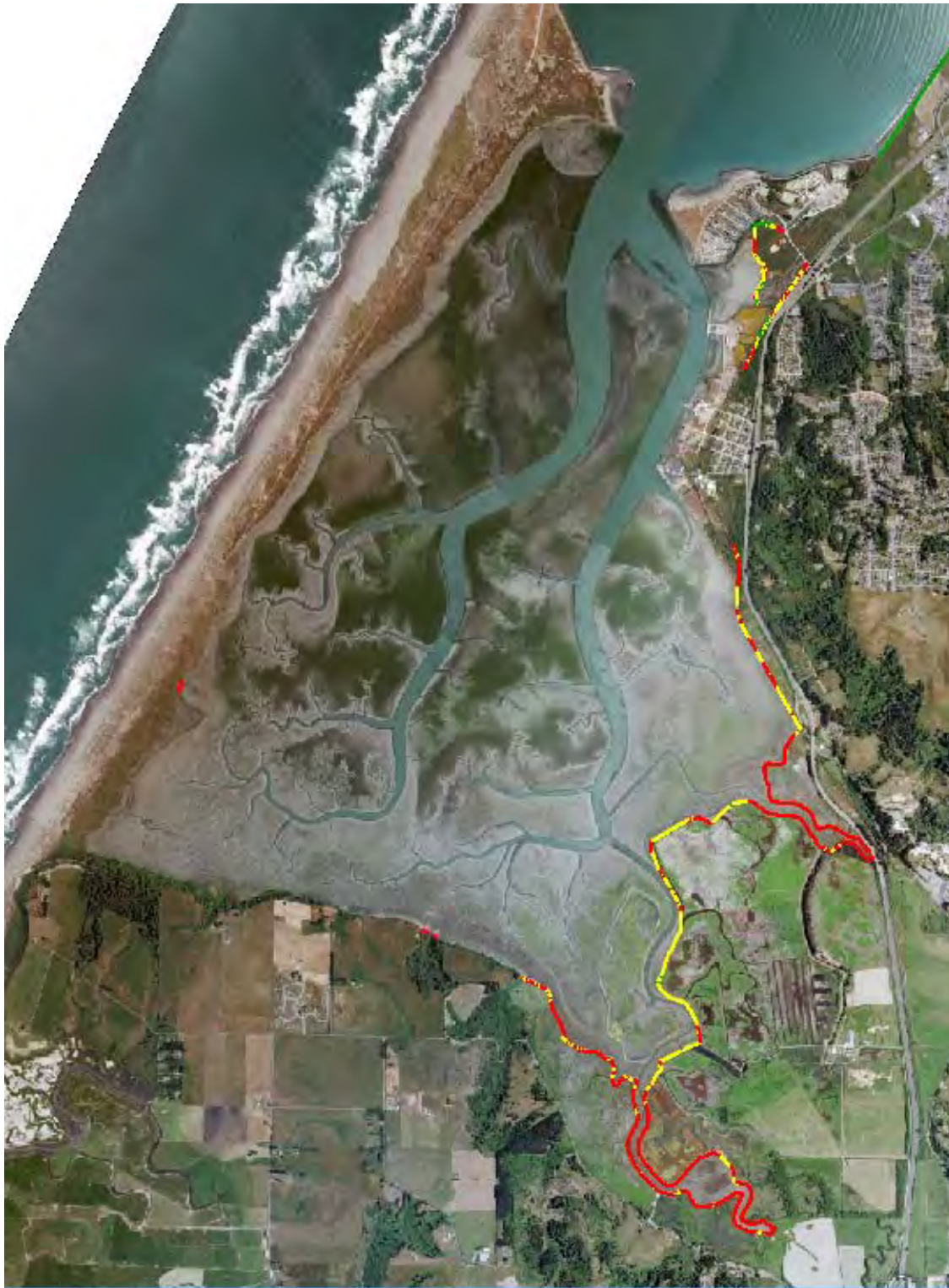
Figure 6. Diked and railroad shoreline vulnerability rating for South Bay; red high, yellow moderate, and green low.
