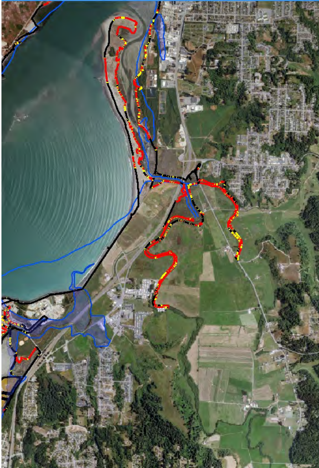
Figure 93. Elk River Slough shoreline areas overtopped by 1 foot of sea level rise (red), and 2 feet (yellow).
