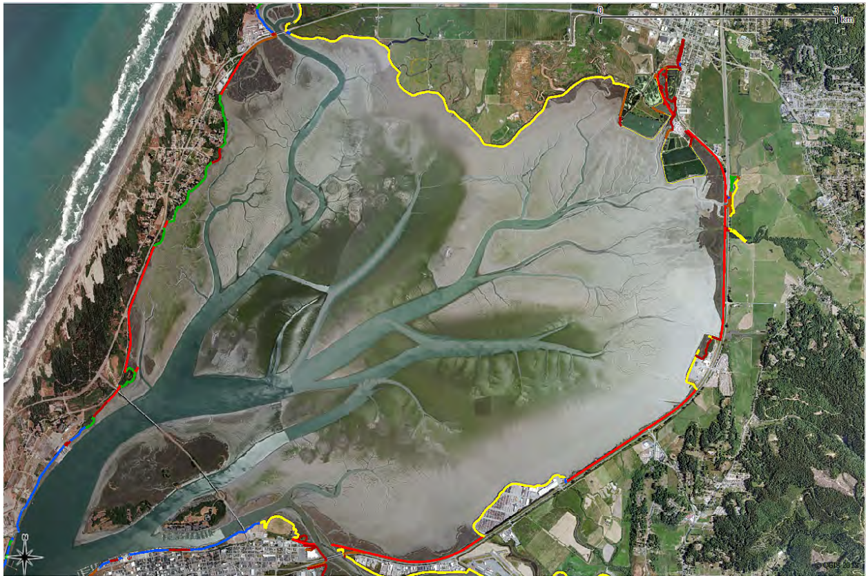
Figure 37. Distribution of shoreline structure types on Arcata Bay: dike (yellow), natural (green), railroad (red), fill (maroon), fortified (blue), and roadway (brown).
