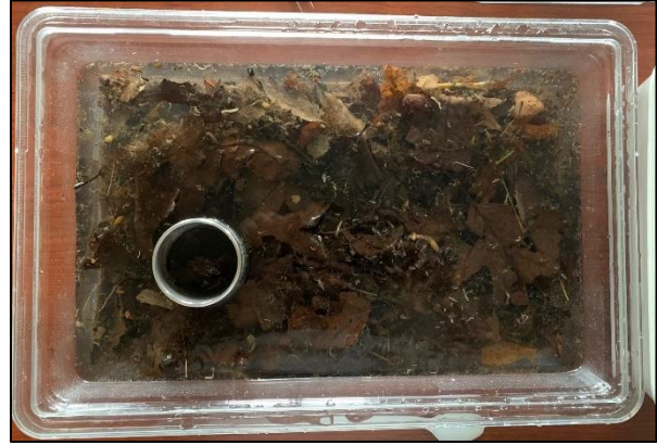
Photo 3. Subsampling pan with sample contents and one “cookie cutter” grid selected.
