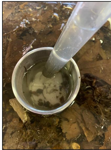
Photos 4-6. Contents of the subsampling grid are removed using spoons, turkey basters, etc.
