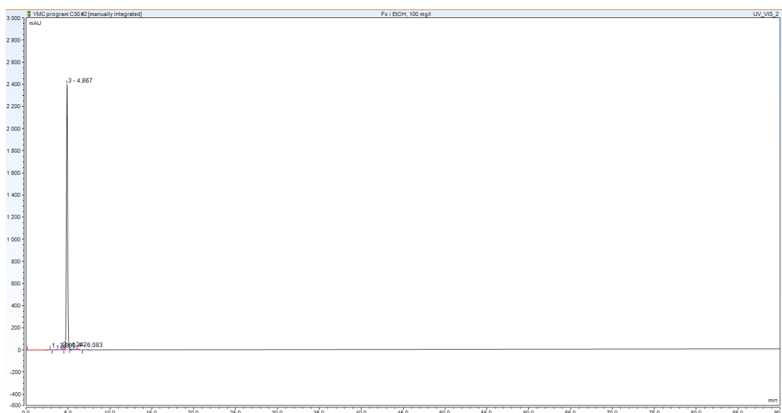
Figure 11 – A chromatogram of unmodified YMC program with 20 \mu l of a 100 mg/l Fucoxanthin standard in ethanol at 450 nm.
