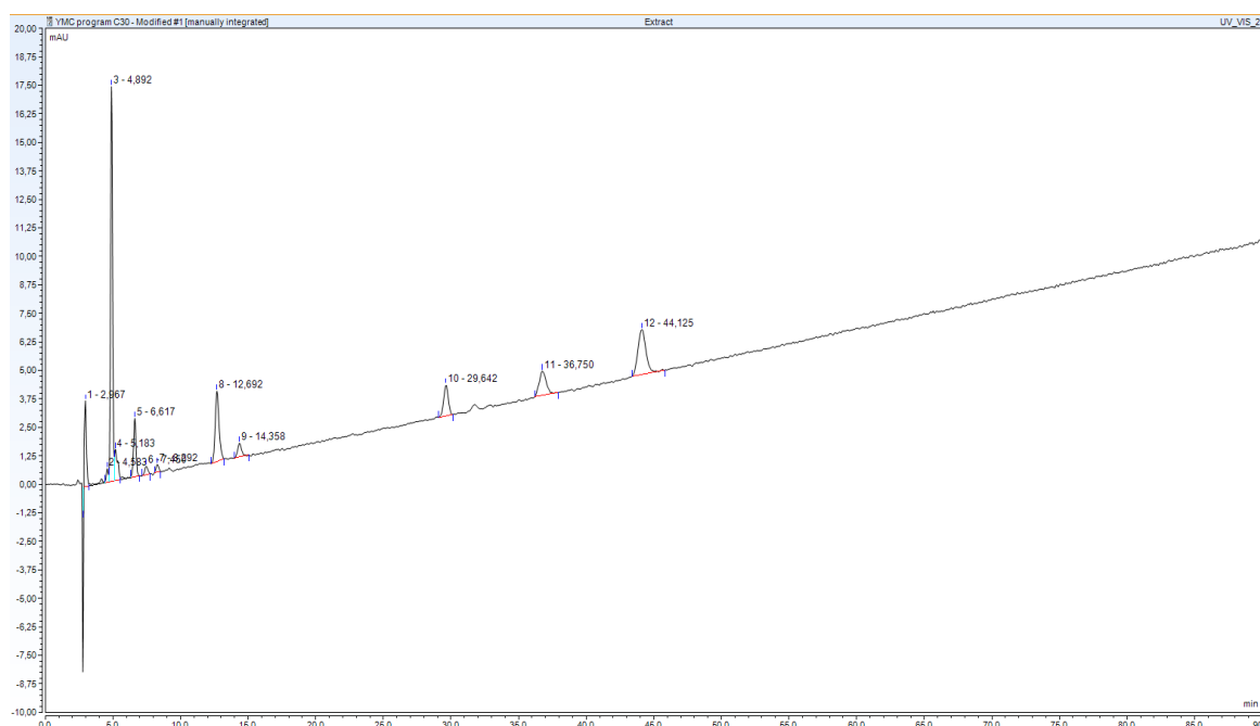
Figure 12 - A chromatogram for the modified gradient program #1 with 20 \mu l of an ethanol extract at 450 nm. The concentration of the extract was about 15 000 mg/l.
