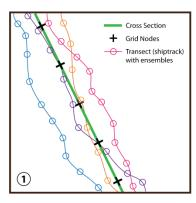
**Step 2.** Project transect data to the cross section plane using an orthogonal translation
