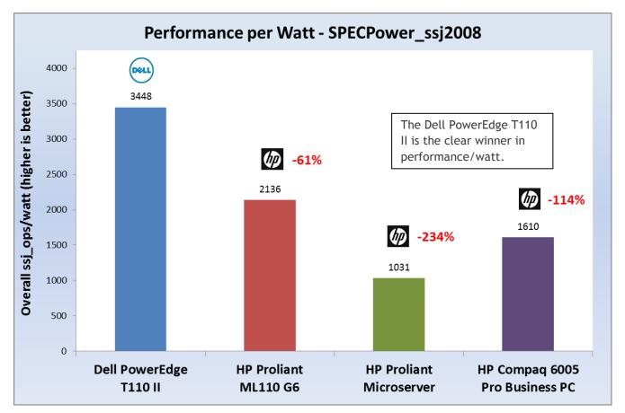
Figure 4: Comparison 3 - SPECpower\_ssj2008 Overall Performance per Watt (ssj\_ops/watt)
