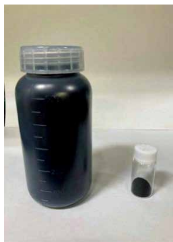
Fig 2. Polymer-wrapped catalyst prepared from industry-scale production (left: 0.1 kg) vs lab-scale synthesis (right: 10 mg).
