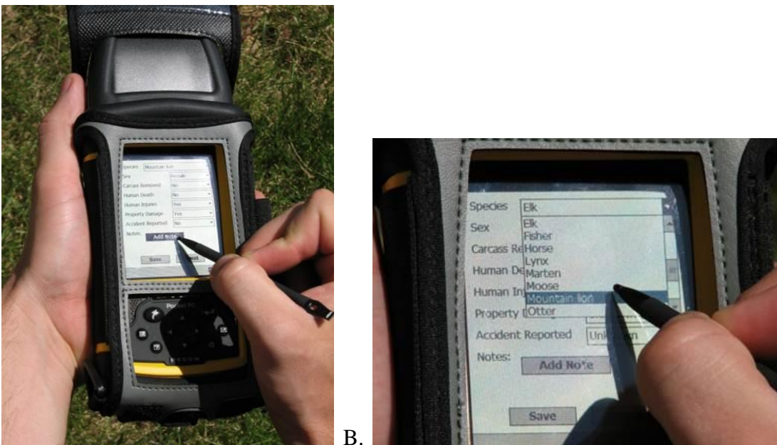
Figure 2.2. Trimble GPS unit (A) and ROCS software (B) used by WDOT maintenance personnel to collect WVC data. (Photos: WTI)
