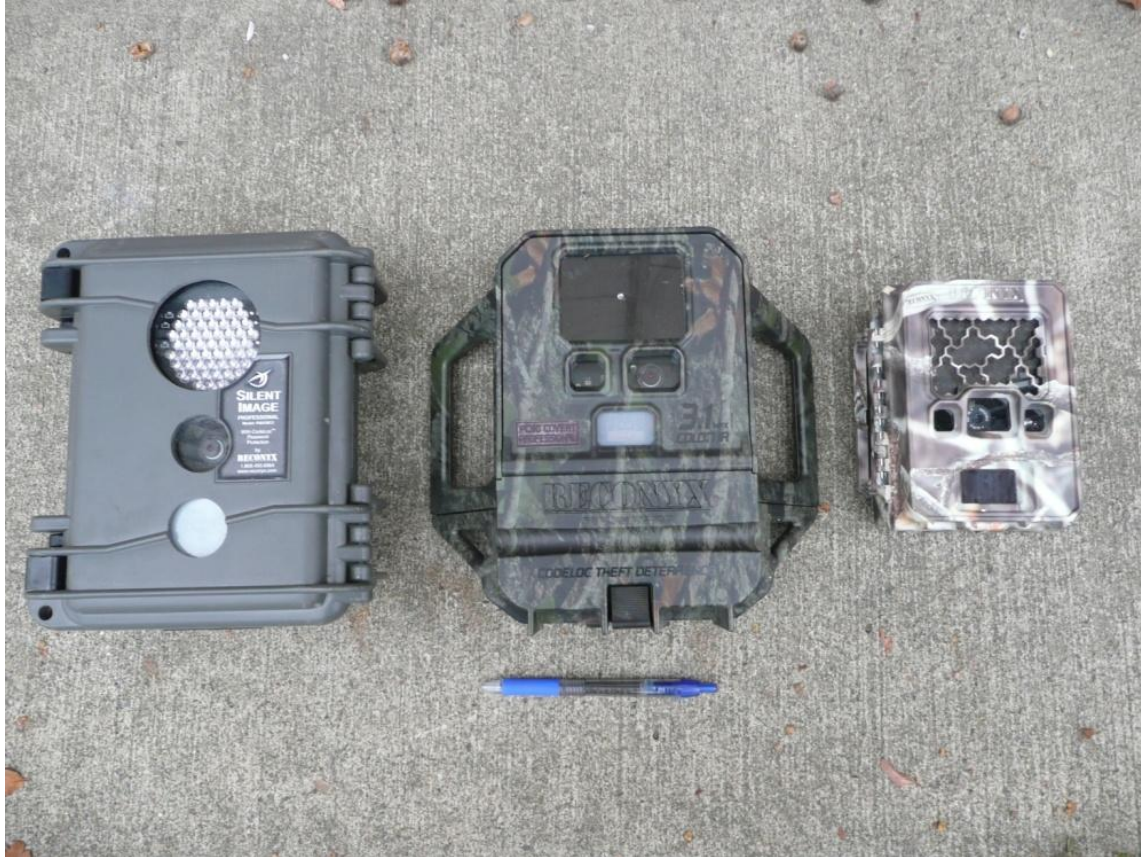
Figure 3.2. Three Reconyx-brand digital remote cameras used to monitor culverts, underpasses, and bridges. Silent Image, Rapid Fire, and Hyperfire models are shown from left to right. (Photo: R. Long/WTI)
