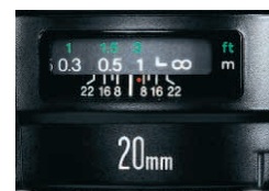
Photo-1 Hyperfocal Length Set Condition
