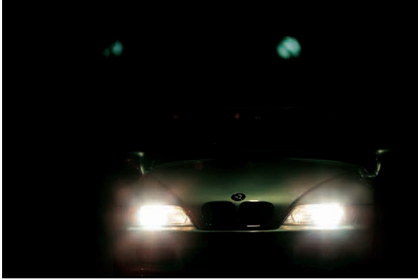
In lenses employing flat protective glass, a reflection occurs between the image sensor and the protective glass, which causes the subject to be photographed in a position different from the actual position.
