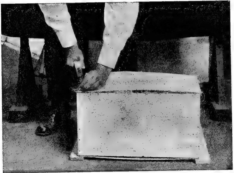
Nailed-down case over cross battens showing bulge top and bottom.
