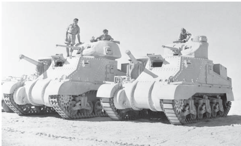
ABOVE • US-produced M3 medium tanks with the British-inspired Grant version on the left and the Lee version on the right, both armed with hull-mounted 75mm guns. (Imperial War Museum, E 14053)
