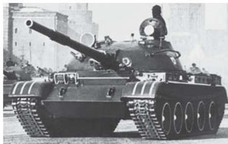
ABOVE • The Soviet T-62 was more than a decade ahead of other tanks in being armed with a high-velocity, smooth bore gun firing APFSDS ammunition with arrow-like penetrators.
