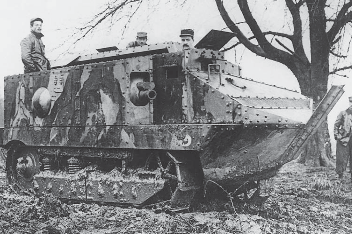
ABOVE • The first French tank built in September 1916 by the Schneider company, after which it was named. (Imperial War Museum, Q 57721)
