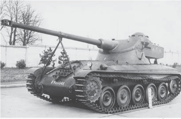
LEFT • French AMX 13 light tank of the early 1950s, the first to have a bustle autoloader for its gun. (French Army)
