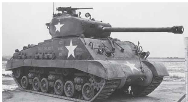
ABOVE • A late M4A3 version of the US Sherman medium tank armed with a 76mm gun that continued to be widely used for several years after the Second World War. (US Army)
