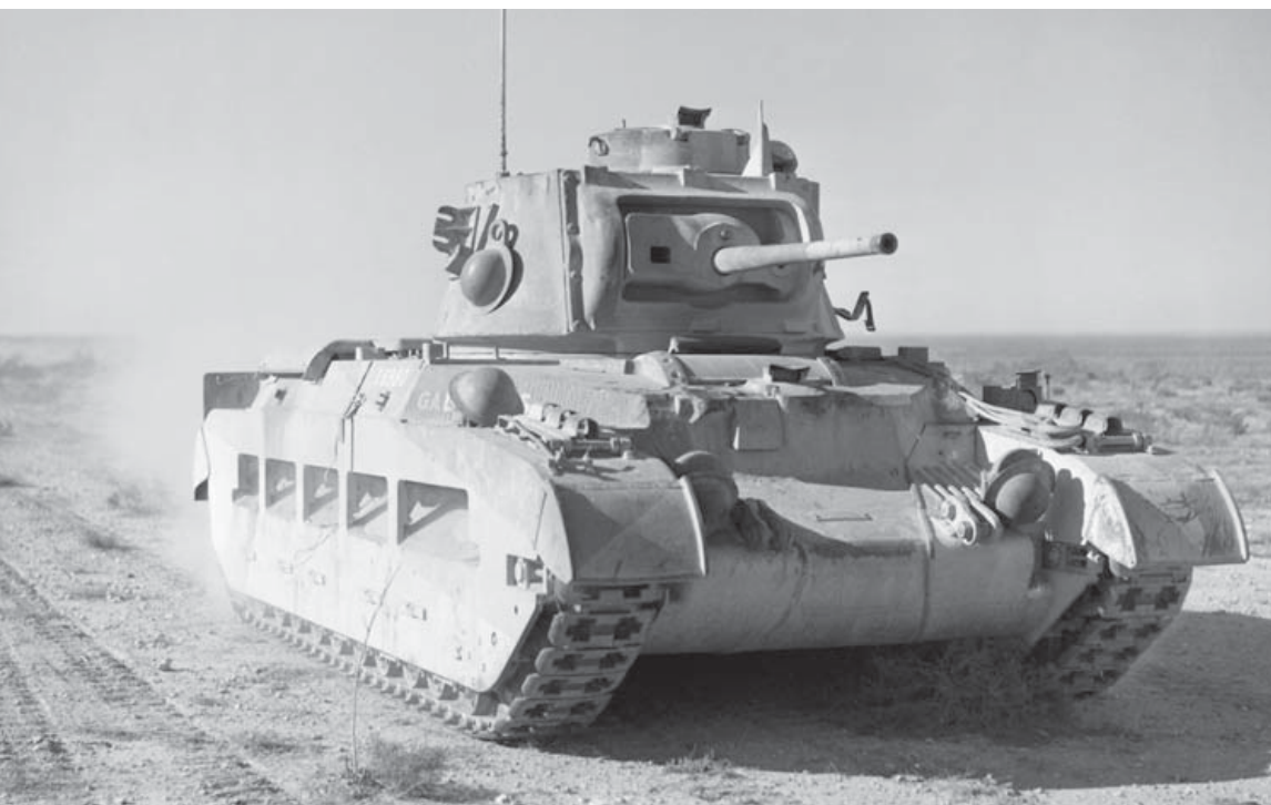
BELOW • The Matilda infantry tank, the most effective British tank in the early stages of the Second World War, due mainly to its thick armour. (Imperial War Museum, E 1416)
