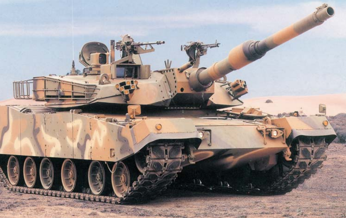
ABOVE • The K1A1, the second version of the South Korean K-1 tank designed in the United States but to a South Korean specification, and, like the second version of the US M1, re-armed with a 120mm Rheinmetall smooth bore gun. (Hyundai)
