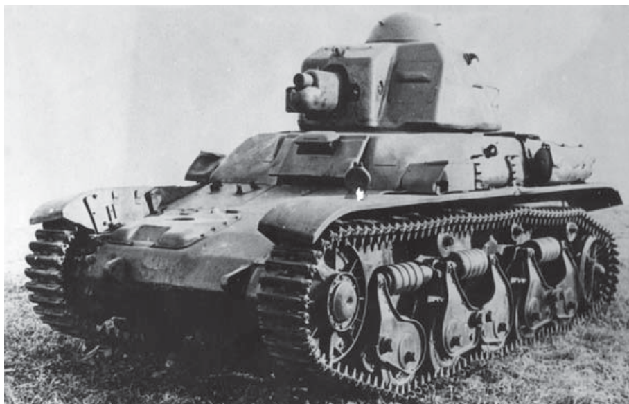
BELOW • The Renault R 35, a relatively well armoured but poorly armed light infantry tank that was the most numerous French tank in 1940.
