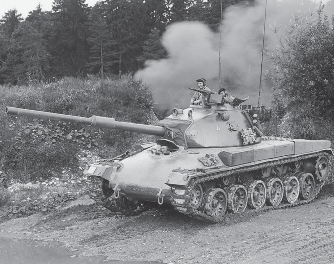
ABOVE • The Swiss Pz.68, a rare example of a battle tank with a hull cast in one piece (Swiss Army).
