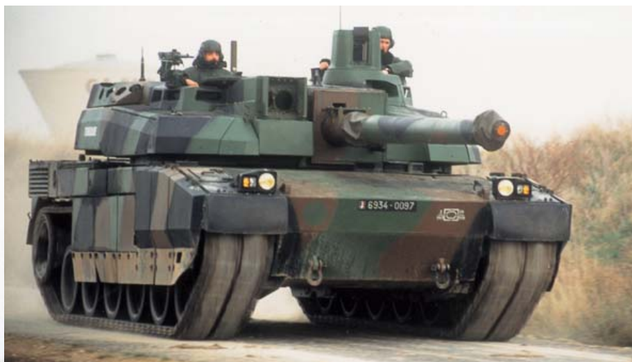
ABOVE • The AMX Leclerc, the last of the third generation of post-Second World War tanks, manned by a crew of three and armed with an automatically loaded smooth bore 120mm gun. (GIAT Industries)
