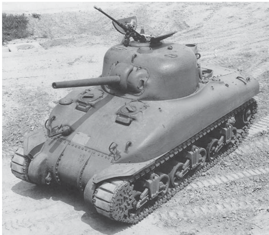
BELOW • An early M4A1 version of the US Sherman medium tank armed with a medium-velocity 75mm gun. (US Army)
