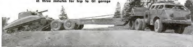
U. S. "dragon wagon" using steel winch-powered cables picks up a disabled tank in three minutes for trip to GI garage
