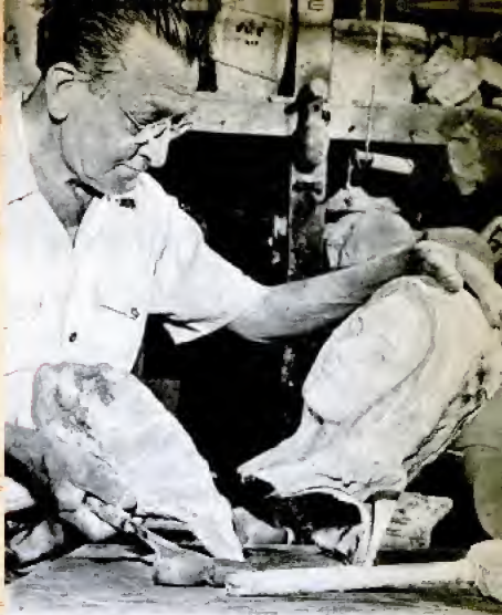
Leopold S. Schmidt breaks mold and inspects face of wax manikin; cast marks will be scraped or melted off
