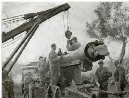
Jeeps or guns, Ordnance kept them fighting: changing a 155-mm. gun tube
