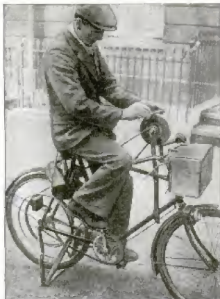
LIFE'S A GRIND to the Briton who coupled the rear wheel of his bicycle to a grindstone with a belt, and travels the countryside sharpening housewives' cutlery. The bicycle lets him cover a wide area and his own sturdy legs provide all the power he needs
