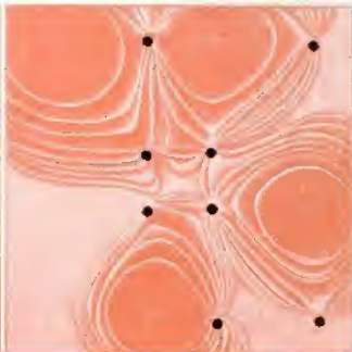
Flow of electric current in electrolytic model simulates flow of oil, gas or water in wells. Photo at left shows wells under study on model. Right, composite photo made on model showing various stages of flooding
