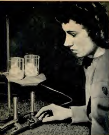
These pictures demonstrate that silicone lubricant withstands higher temperature than petroleum jelly. Left, silicone lubricant is in the left-hand vessel; petroleum jelly in the other. Right, flame melts the jelly
