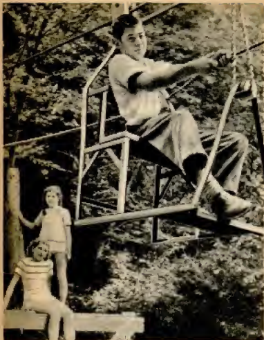
CABLE CAR built by Philip J. Kirst of Kenmore, N. Y., carries him across a gully to get firewood for his parents' weekend cabin. Car will support 500 pounds
