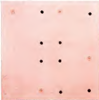
Flow of electric current in electrolytic model simulates flow of oil, gas or water in wells. Photo at left shows wells under study on model. Right, composite photo made on model showing various stages of flooding
