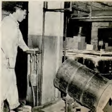
LIFTING 1000-pound drums—a back breaking job—is performed by an air lift. The equipment consists of a double-acting cylinder hoist and three-way valve
