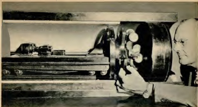
A research man examines model of tunnel digging machine that uses electric motors to operate cutting heads
