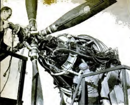
First gas turbine engine to drive an airplane propeller and generate jet propulsion. Below, drawing shows how the G-E Propjet fits into wings of a plane.
