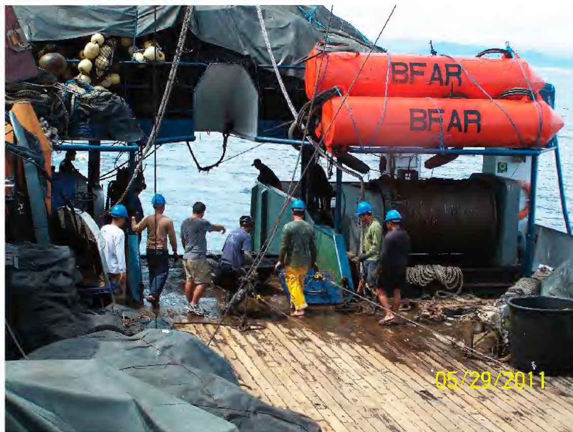
FIGURE 3. The otter trawl during haul-back, otter doors on deck; note beam trawl on right behind black plastic tub.
