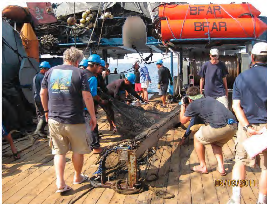
PHOTO 6. Bringing the beam trawl aboard the MV DA/BFAR . Photo by M. Burke.
