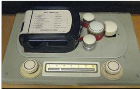
Figure 8. Futuristic at the time... this bar-graph like tape lapse indicator. Source: Google images.
