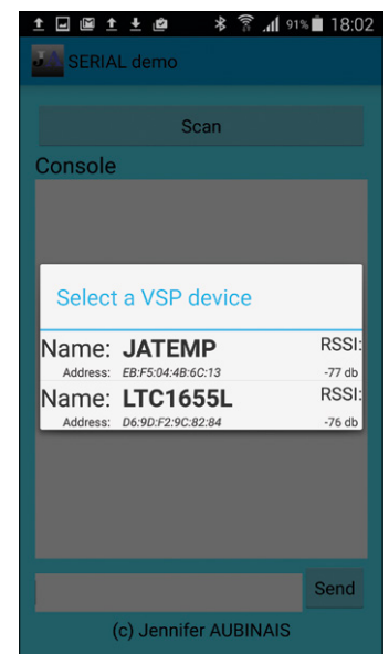
Figure 6. Display of the mDialogFoundDevices Dialog class with two peripherals.
