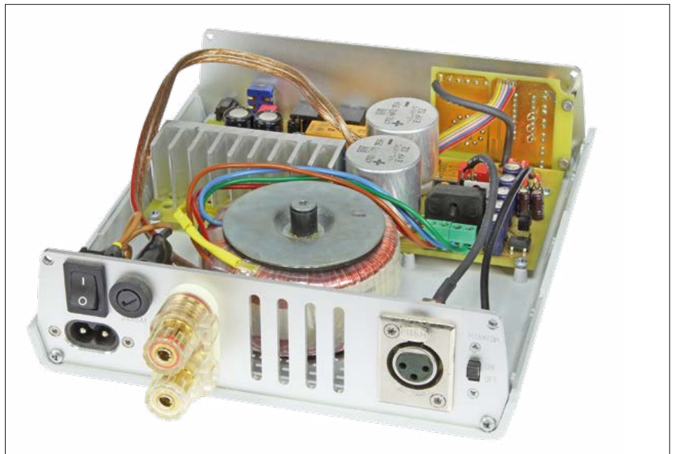
Figure 10. The fully assembled MEASSY, ready to use.
