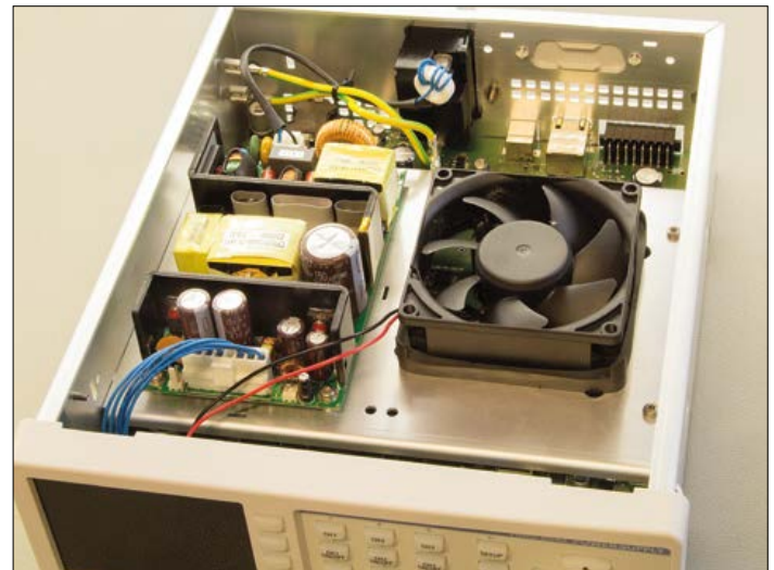
Figure 7. Inside the case. On top is the Cincon 200-W open frame AC/DC switch mode regulator supplying 48 V to the three microcontroller-controlled DC/DC converters on the lower board.
