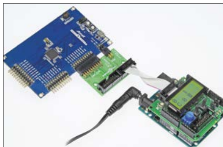
Figure 4. Here we have a SAM D20 board and an Arduino Uno (with extension shield) connected for working together. Because the two polarizing keys of the ECC connectors point outwards on each of the boards, we need to use a 'crossover' ribbon cable.
