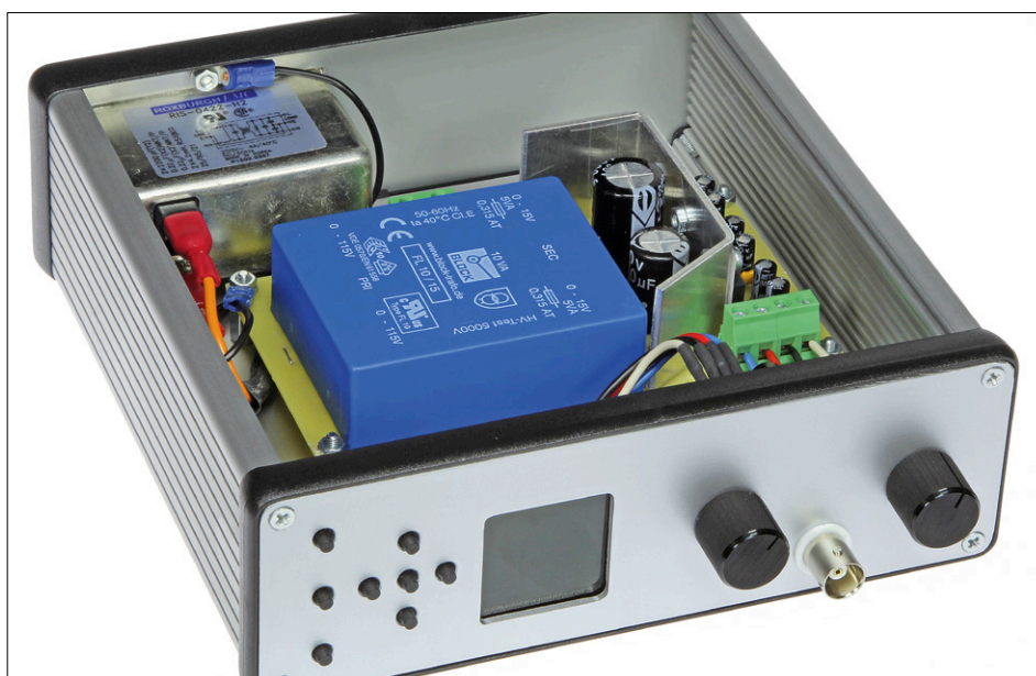
Figure 8. The prototype built at Elektor.Labs by Jan Visser. All cutouts were done with a 100- \mu CNC machine simple tools, care & patience.
