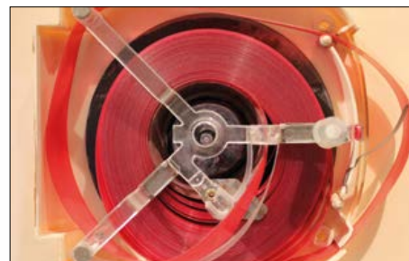
Figure 4. The clever tape jam inhibitor in the Tefifon KC 1 cassette.
