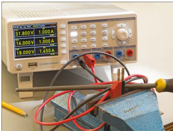
Figure 4. The Pease Test — there were sparks but it survived.
