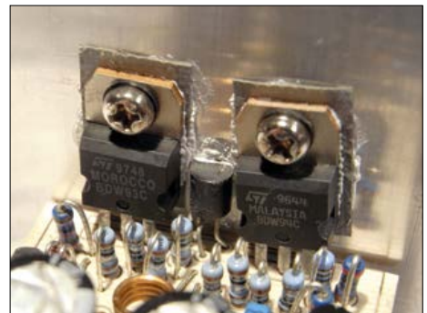
Figure 6. Low in aesthetics but definitely okay for keeping the power transistors cool.
