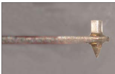
Figure 6. Macro image of the KC 1's pickup stylus.
