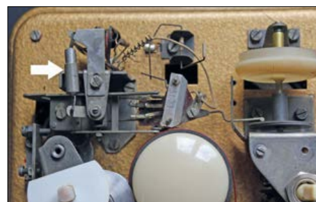
Figure 7. Stylus landing damper (white arrow).
