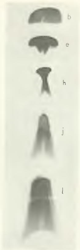
Fig. 2. Photographs showing the distribution of light at different planes in a beam of light passing through a focal region. The lettering is the same as in fig. 3.
