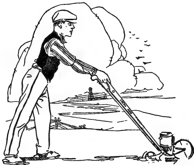
FIG 12.—The wrong way to push a seeder or hand-cultivator. It is almost impossible to control the direction of the machine and the operator tires quickly.
