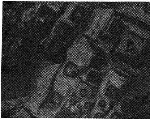
Fig. 3 X 350 Etch pattern on (010) cleavage of the crystal etched in Methanol for two minutes.
