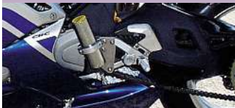
Slimline & Powerful Electronic Actuator replaces the function of your foot
