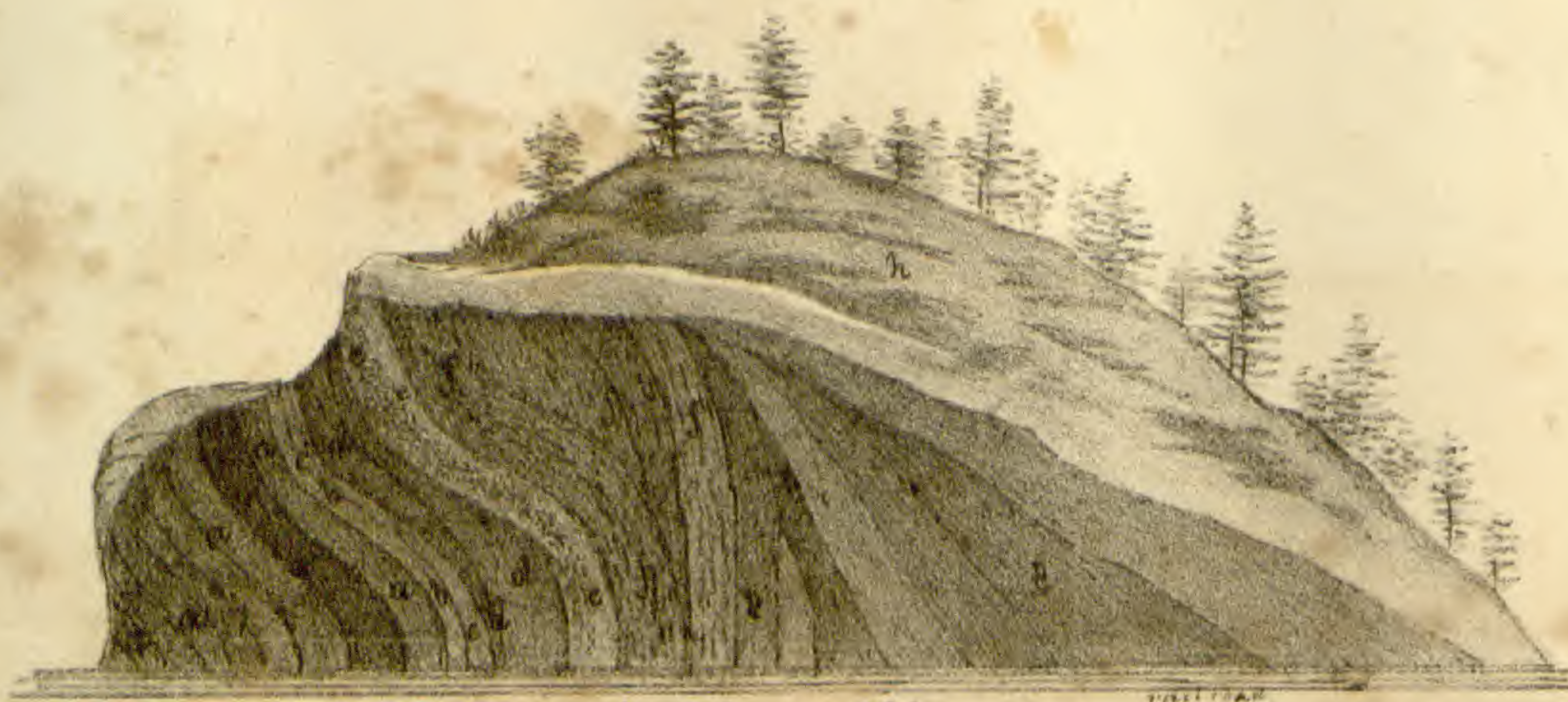
Vertical section at W. side of Avenue No. 3 a. good coal—b. slate & broken coal.—c. yellow & black slate. d. good coal. — gray wacke filled with numberless vesicles of various sizes. f. broken gray wacke in laminae—g. gray wacke firm & broken of very fine quality h. earth.
