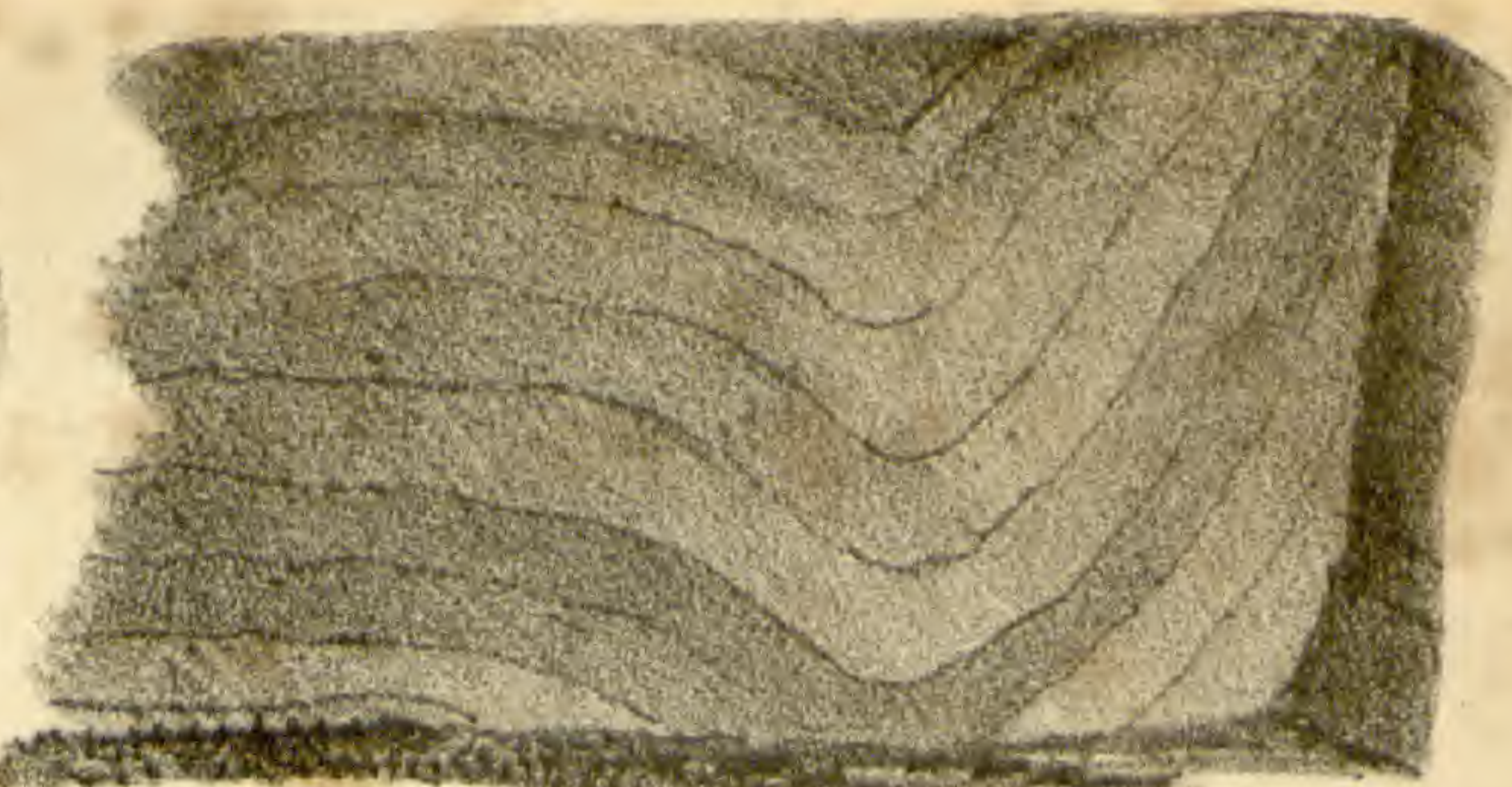
Vertical section at Avenue No. 4. This is good coal throughout, They have cut into the mountain in spots ranging with this to an extent of 3 miles & find the stratification at all of them exactly similar.
