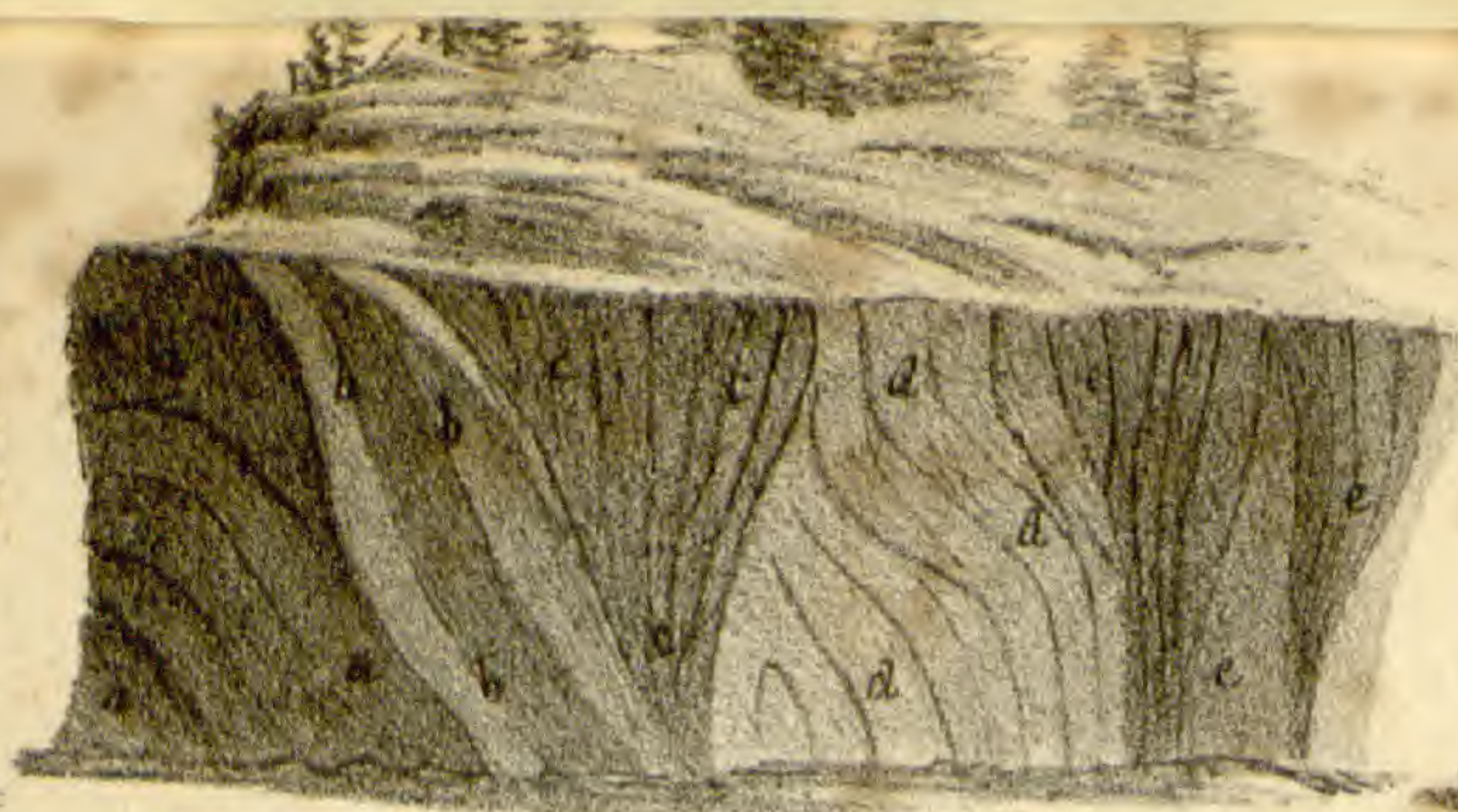
Vertical Section near Avenue No. 3. a. good coal. b. broken coal. c. Soft black slate. d. Yellow slate. e. pretty good coal.
