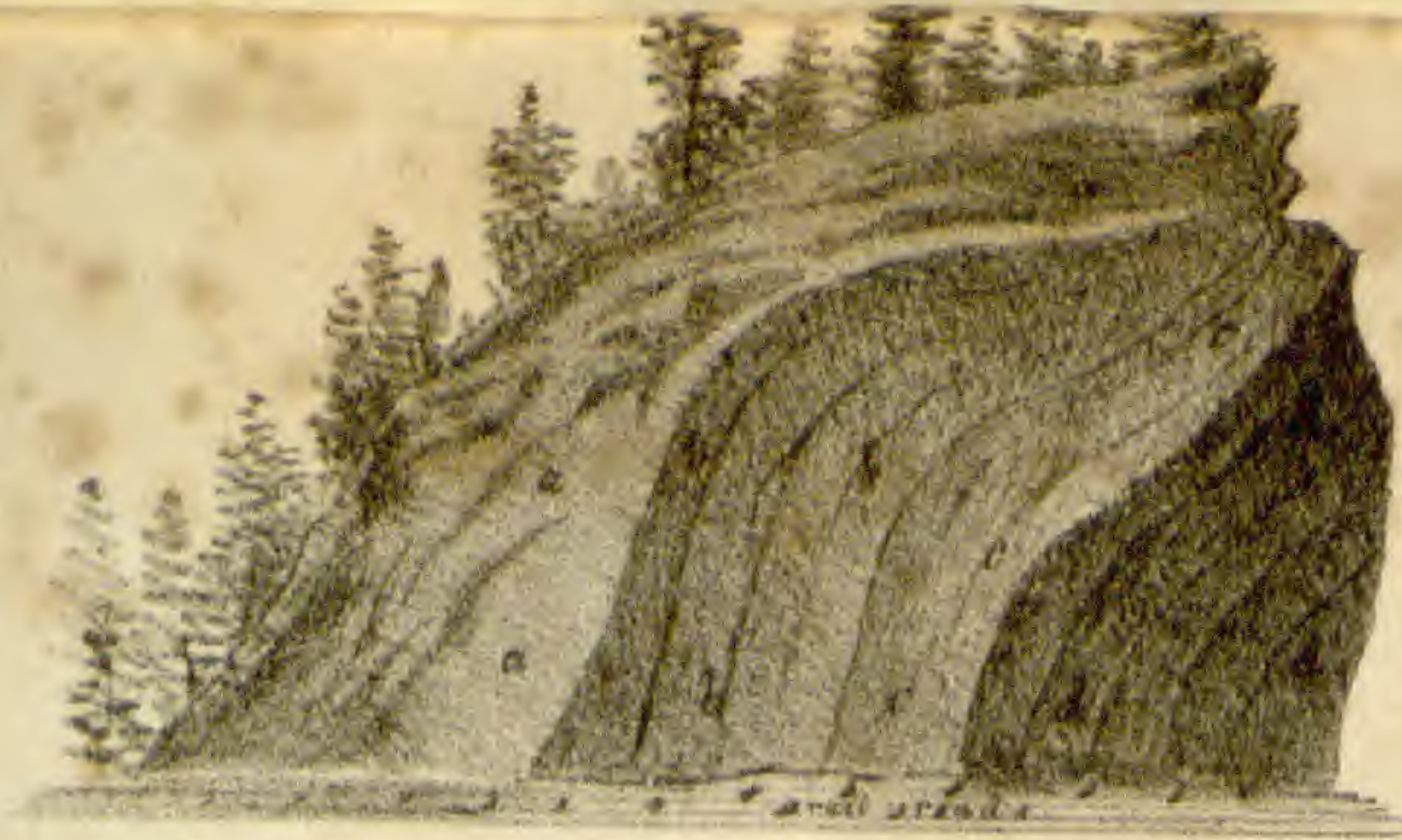
Vertical Section at Avenue No. 2. a. earth & loose stones. b. gray wacke. c. broken coal & earth. d. good coal.
