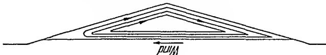
Fig. 163. Sketch of NAKANO'S experiment showing the establishment of vertical currents. After NAKANO 7
