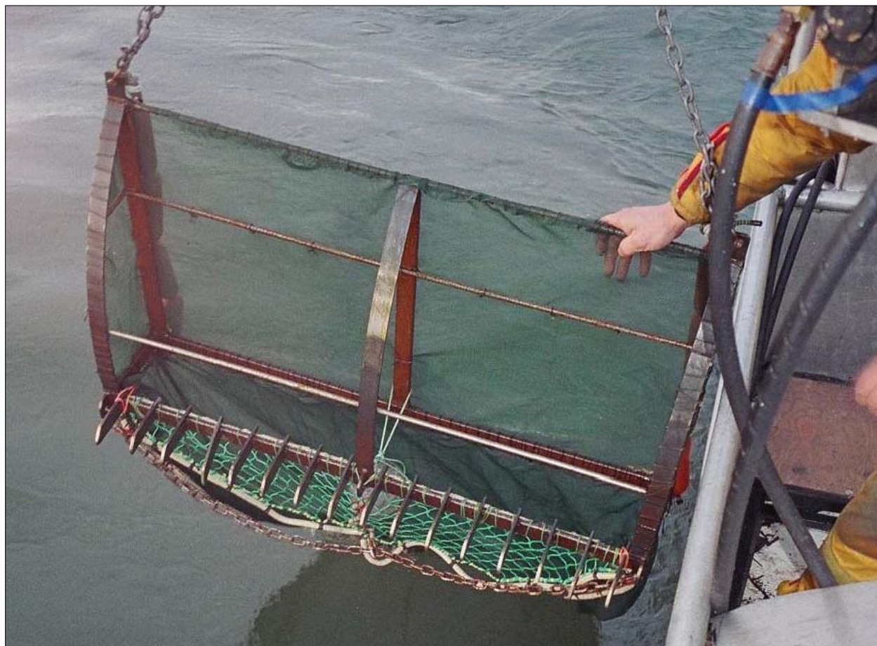
Figure 16 Photo of Rake Trawl (Taylor and Perrin 2005)
