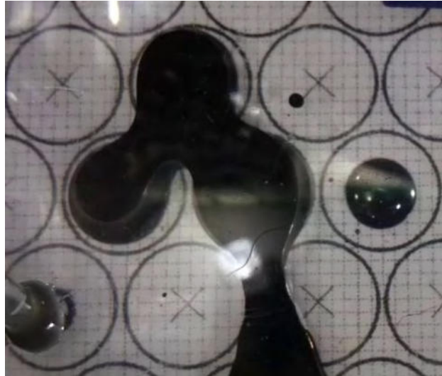
Figure 3 PAPELL Experiment area 1 in-orbit example footage: Transported ferrofluid on multiple active electromagnets and a single separated droplet. A circle has a diameter of 10 mm.
