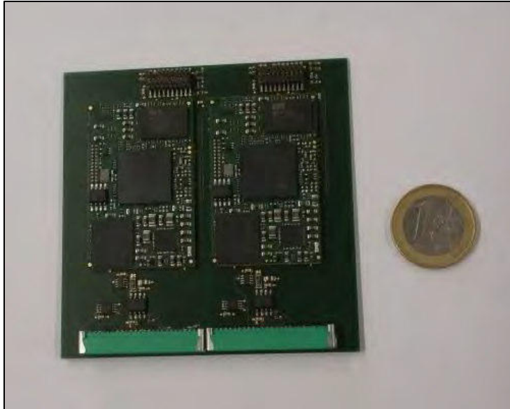
Figure 2. ADIA-Light onboard hardware module consisting of two BeagleCore BCM1.STR modules (AM335x CPU).
