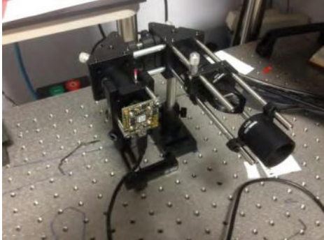
Figure (1): CHAFF bench-top prototype with the CMOS sensor on the spectral arm.
