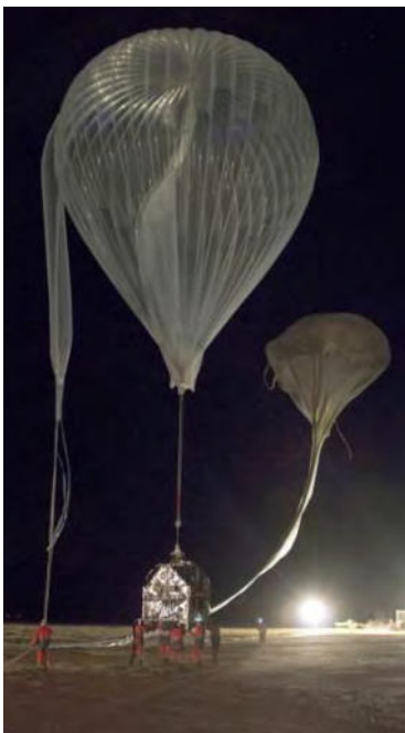
Figure 5. Launch methods - Left panel: Launch with auxiliary balloon (CNES) – Right panel: Launch with Hercules vehicle (SSC)
