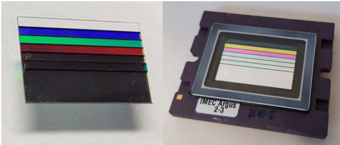
Figure 5: 7-band assembled glass filters before (left) and after (right) direct integration onto the multi-band CCD-in-CMOS TDI imager
