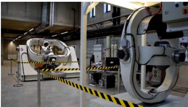
Fig.7: The high precision, high dynamics turntables to characterize in hardware-in-the-loop-tests intersatellite links and coordinated pointing control in observations.
