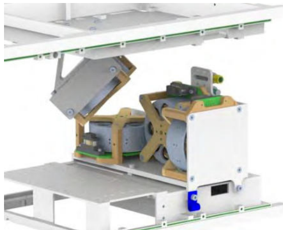
Figure 6. Configuration of the four reaction wheels.
