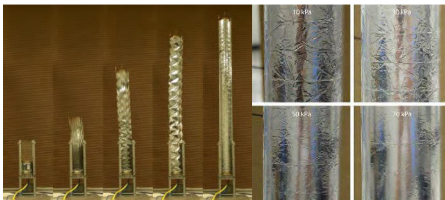
Fig. 4. (left) The Inflatable Cylindrical Mast Deployment Sequence; (right) Residual Creases after Depressurisation from Different Inflation Pressures (10–70 kPa)
