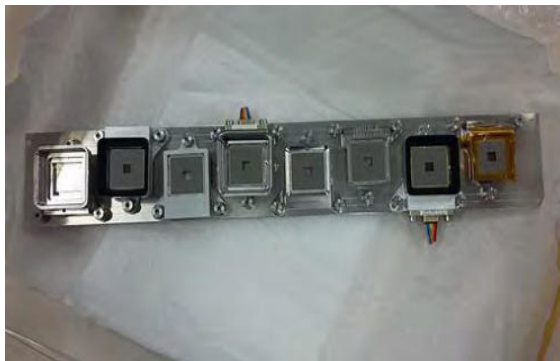
Figure 4: thermal cycling glue samples
