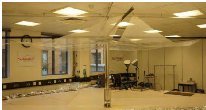
Fig. 5. InflateSail Inflatable Mast and Drag Sail Deployment Test
