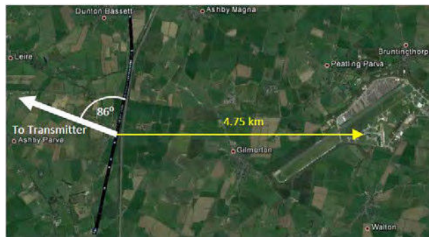
Fig. 6. Satellite Image (Bing Maps) of the Bruntingthorpe Target Area with the Flight Path of the Aircraft (black line), Distance and Direction to the Transmitter (white line), and the Distance to the Airfield (yellow line) Shown
