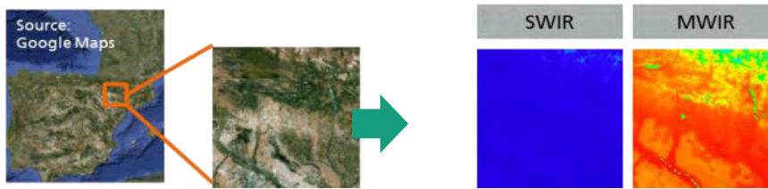
Figure 2: Exemplary representation of the FOV of a satellite-based sensor in SWIR and MWIR. The spectral background image was calculated using the atmospheric model MATISSE. It can be seen that in the SWIR the earth's background signal is strongly absorbed by the atmosphere, while the surface structure in the MWIR is still recognizable. Both figures have the same scaling.
