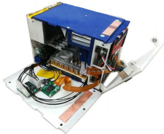
Figure 2 PABELL Flight model prior to final close-up and sealing for ISS operation[6, 7].
