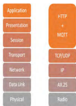
Figure 6 Groundstation Network OSI-layer model
