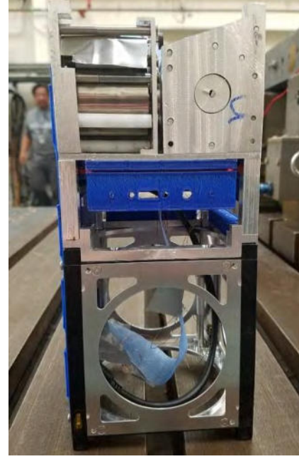
Figure 3. Prototype of DMD with CubeSat Structure
