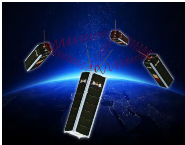
Figure 1: NetSat formation demonstrating precision orbit and attitude control and inter-satellite communication.
