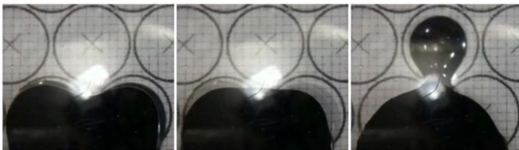
Figure 4 PARELL Experiment area 1 in-orbit example footage: Overspill transfer example. Frame 1: two lower electromagnets are active, negative curvature bridge in between. Frame 2: Negative ferrofluid curvature relief, top electromagnet active Frame 3: Transfer of ferrofluid.
