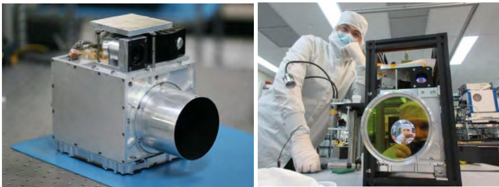
Figure 2. GHGSat-D fully integrated payload (left) and GHGSat-C1 payload (right).
