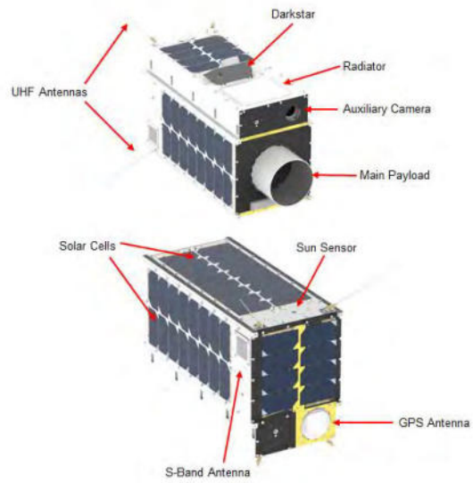
Figure 5. GHGSat-C1/C2 exterior solid model.
