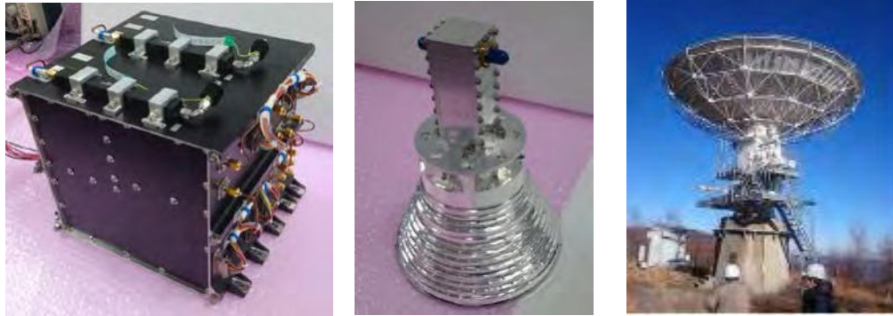
Fig.4 Left : High Speed X band Transmitter. Center : Medium Gain Antenna (MGA). Right : 10m Ground Station Antenna
