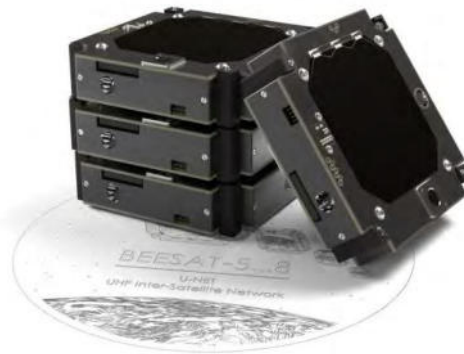
Fig. 3: Picosatellites BEESAT-5 to -8 of TU Berlin with a precise onboard orbit determination module and inter satellite link
