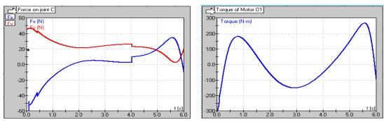
Figure 6 Reaction force on joint C and Transmitted moment – Torque of motor on joint O<sub>1</sub>.
