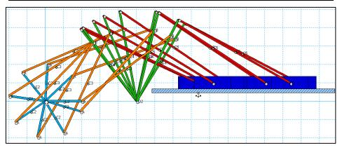
Figure 7 Different positions (9 trucking frames) of mechanisms during the motion
