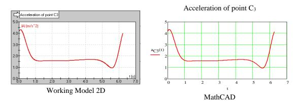
Figure 5 Acceleration of point C<sub>3</sub>
