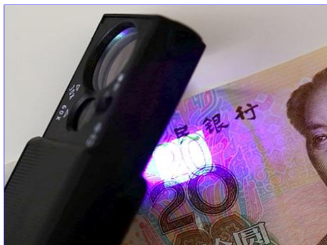
Fig. 11. 380 nanometer UV LED in money checking machines.
