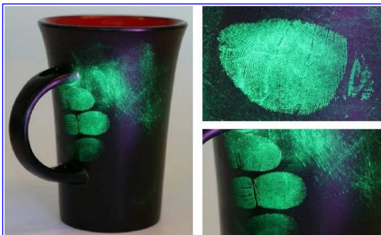
Fig.12. Fingerprints in ultraviolet light, invisible in normal light.
