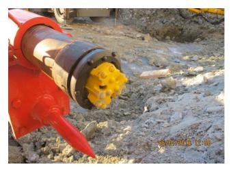
Figure 12: Drill head for steel pipes. Only the yellow drill part is retracted
