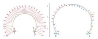
Figure 8: Critical load case, normal force left, bending moments right.
