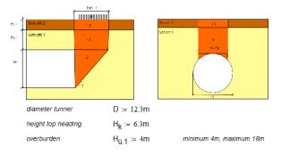
Figure 7: Geometry of failure wedge
