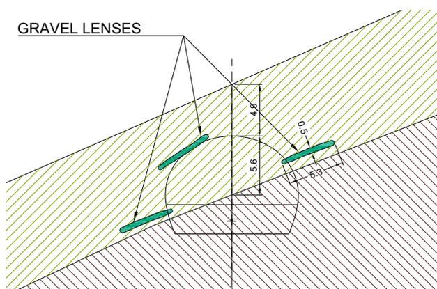
**Figure 6: Gravel lenses at CS 1**
