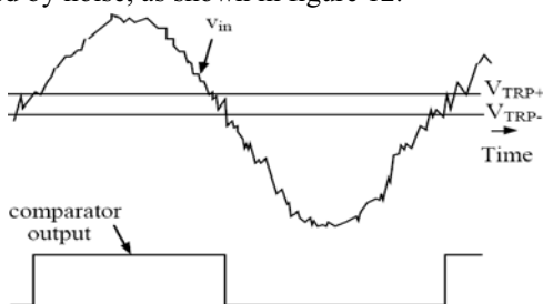
Figure12. Comparator response to a noisy input when hysteresis is added
