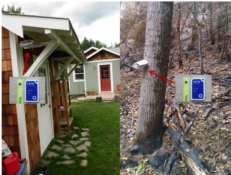
Air temperature data loggers were placed in radiation shields to avoid direct sunlight and subsequent temperature bias.
