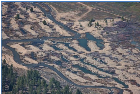
Low altitude aerial photo of dredge mine tailings along Grimes Creek, showing narrow bands of floodplain and discontinuous, degraded riparian habitat. Photo courtesy of Trout Unlimited.
