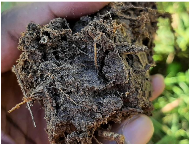
Photo 7: Soil sample extracted from the wetland habitat. Note the grey matrix and low chroma soil mottles which indicate prolonged soil saturation.
