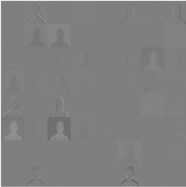
Figure 7. Features visualisation of the first convolutional layer
