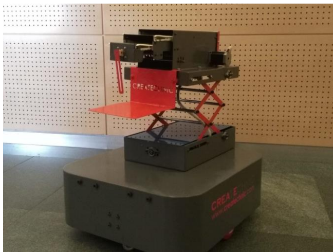
Figure 5. A prototype of a warehouse robotic arm for gripping and moving standardized containers
