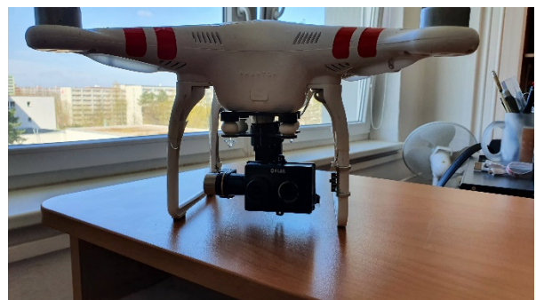
Figure 4. Duo DJI Phantom 3 drone, with external FLIR Duo thermal camera.
