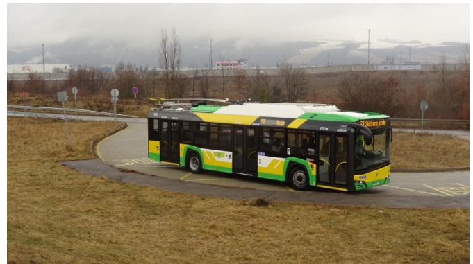
Fig. 1. Battery-assisted trolleybus used in Žilina on road with no overhead contact lines [3]
