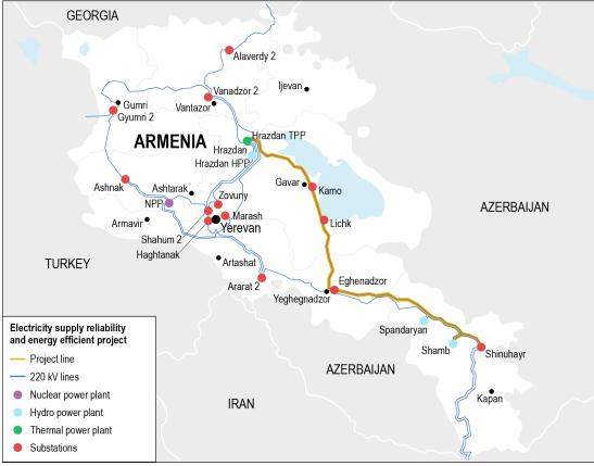
Figure 5.8 Armenia's electricity transmission system
