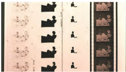
FIGURE 10. Film strips: Foreground line, foreground 1 matte, foreground 2 matte combined in the optical printer.
