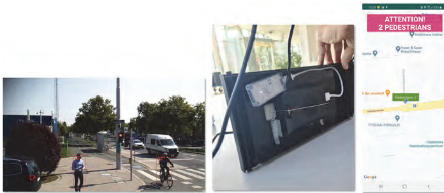
FIGURE 1. (a) Object detection. (b) Traffic light with the camera and Raspberry Pi. (c) App with the alert about the object in the dead corner.
