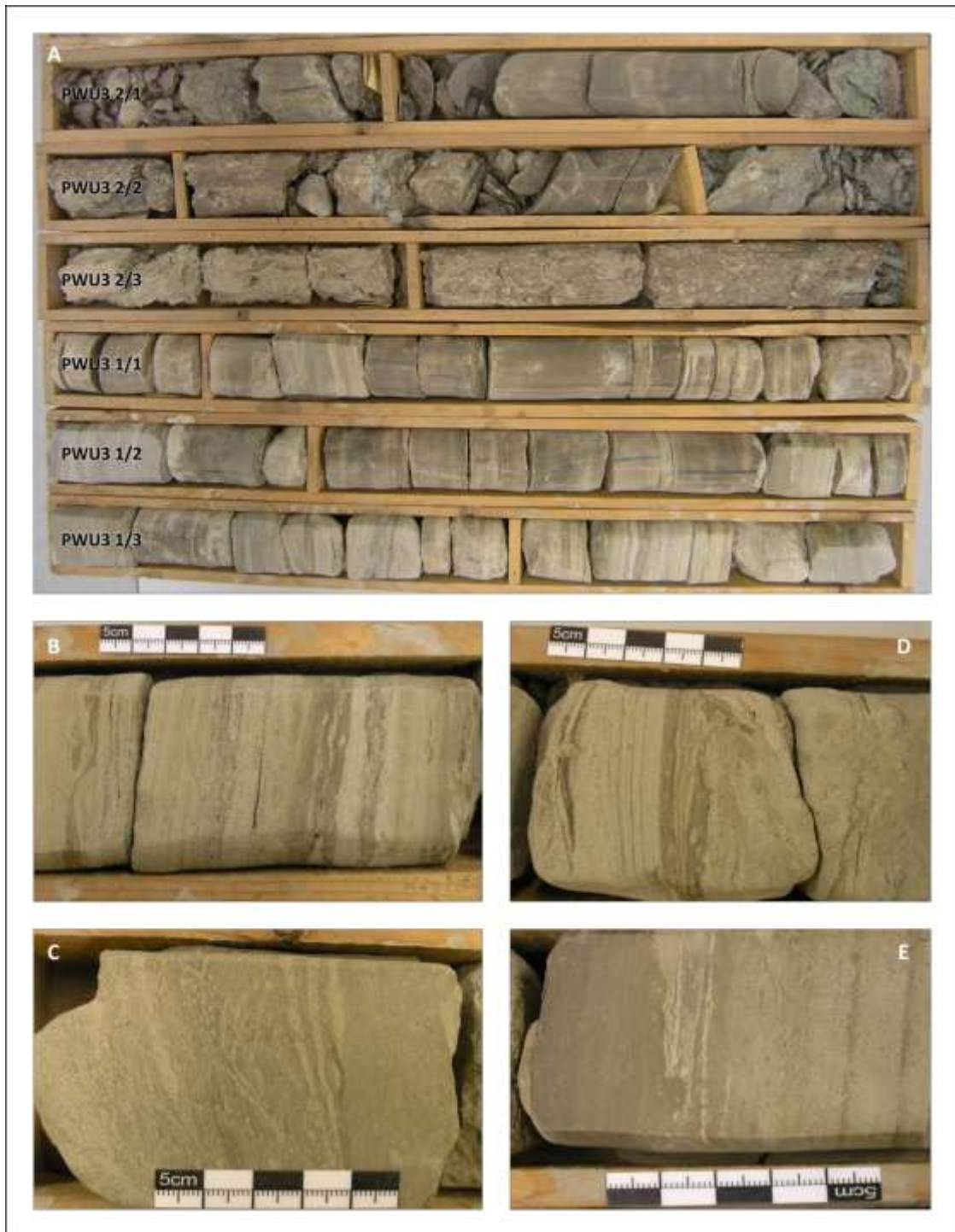
Fig. 43: A: View on cores PWU3 (1123–1128m) 1 and PWU3 (1438–1443m) 2. Core PWU3 (1123–1128m) 1 comprises brownish, bedded sandstone, which grades downcore into clayey silt. One box measures one metre in length. B-D: Detailed views on examples for laminae, thin layers of carbonised plant remains as well as fine ripple structures, cross bedding and intercalations of darker clay in core PWU3 (1123–1128m) 1/3. E: Similar features found in core PWU3 (1123–1128m) 1/2.
