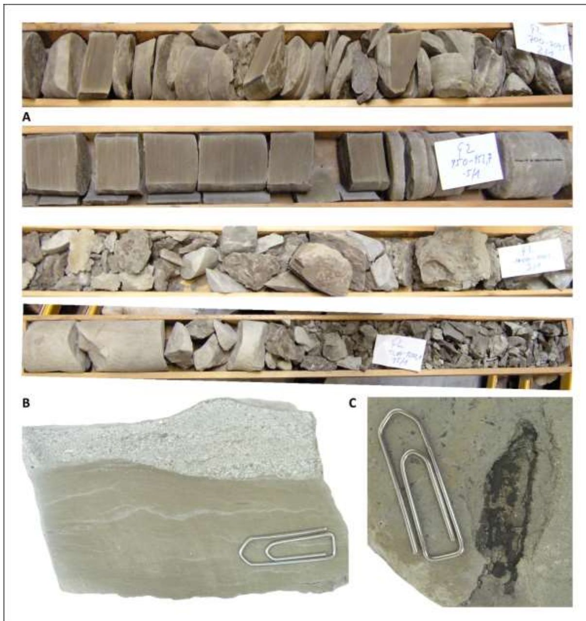
Fig. 16: A: Core GI2 (700–704.5m) 2/1 at the top comprises greyish, micaceous sand. Second core GI2 (950–952.7m) 5/1 is composed of brown-grey laminated marl, whereas the third one GI2 (1000–1002m) 7/1 shows greyish, fine sandy marl. Core GI2 (1200–1201m) 15/2 at the bottom contains light grey homogenous sandstone (left) and darker, more clayey marl (right). One box measures one metre in length. B: Detailed view on a piece of core GI2 (1084–1086.7m) 10/1 with changing lithology from light grey sandstone to brown-greenish, sandy marl. C: Carbonised plant fragment found in core GI2 (1125–1126.6m) 12/1.
