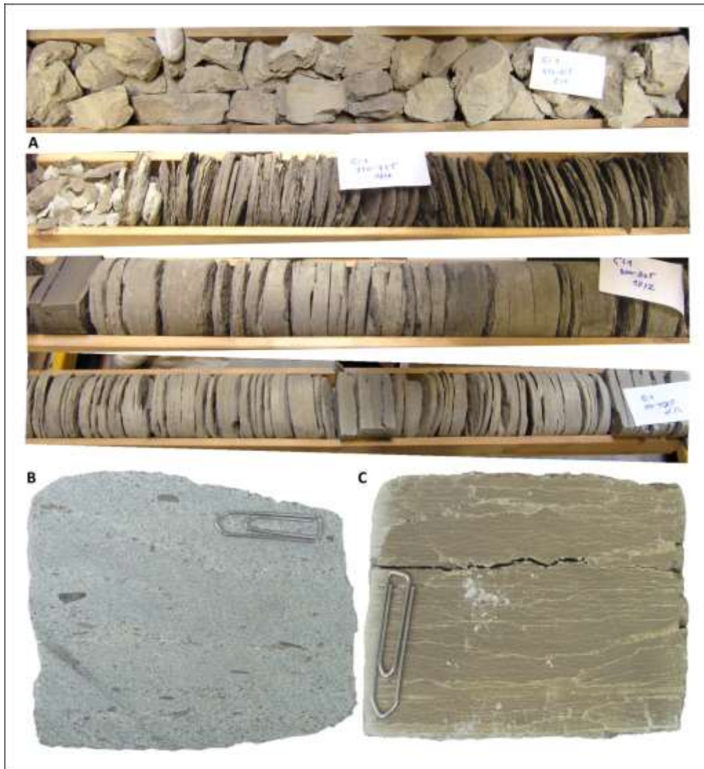
Fig. 13: A: Characteristic lithologies of different cores of the Ginzersdorf 1-well. The uppermost core G11 (450–455m) 5/1 contains silty fine-grained sandstone, whereas the second one G11 (750–755m) 11/1 is composed of brownish, laminated marl. The following core G11 (800–805m) 12/2 comprises micaceous, fine sandy marl. Core G11 (950–953.5m) 15/2 at the bottom shows greyish fine sandy marl with lamination. One box measures one metre in length. B: Greyish sandstone found in the lower part of core G11 (999–1003.7m) 16/1. C: Detailed view on dark brownish laminated marl of core G11 (700–705m) 10/3.
