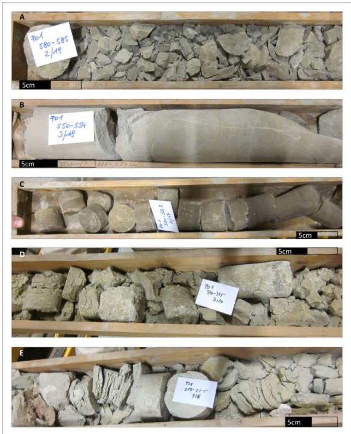
Fig. 47: A: View on the green-greyish marl of core PO1 (580–585m) 19/2. B: Homogenous greyish marl in core PO1 (550–554m) 18/3 C: Core PO1 (520–525m) 17/2 with more brownish marl. D: Top view on greenish marl of core PO1 (310–315m) 10/2. E: Greyish fine sand of core PO1 (250–255m) 8/1.
