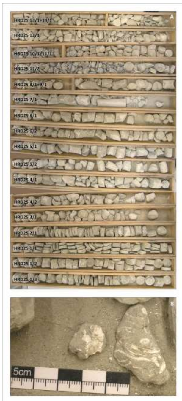
Fig. 25: A: Fine- to middle-grained sand in cores HRD25 (290–298m) 1 to HRD25 (979–984.5m) 14. One box measures one metre in length. B: Mollusc remains found in core HRD25 (645–650m) 7/1.
