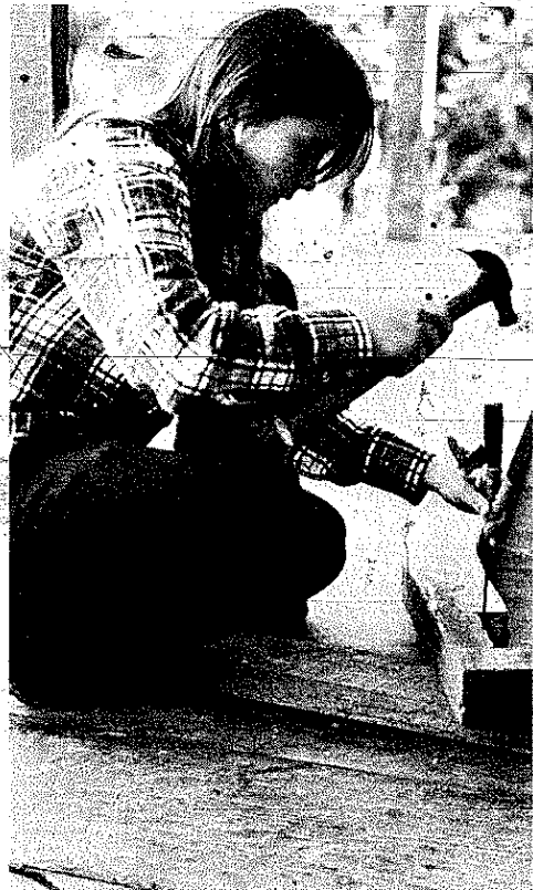
PLATES 162-163 Tedra begins his sleds with the runners which, in this case, are made of cucumber. Here, Cheryl Stocky cuts the notches that the front crosspiece will fit into.
