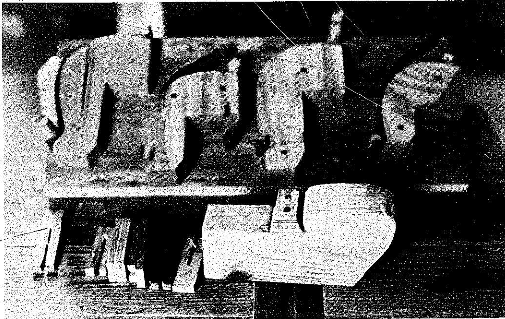
PLATE 115 The "ribs" or sides of the fiddle are thin strips of maple \frac{1}{4} " wide, and are soaked in hot water until pliable and then placed in wooden forms to harden in the correct shape. Blocks of maple— \frac{1}{4} "-high—are placed at each end of the top to hold the ribs secure (see Plate 120)
