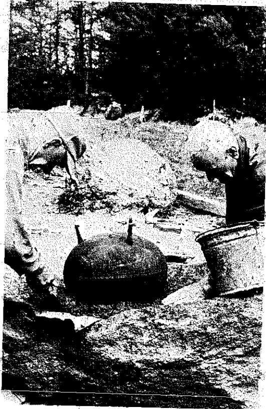
PLATE 257 The clay was then packed around the rim of the pot to keep the flames from the fire that will be built over the pot from lapping in under the rim and setting the wood inside on fire. The piece of tin keeps the mud from filling the groove in the rock and blocking the flow of resin.
