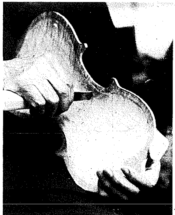
PLATE 129 Garrett shapes the inside concave surfaces and the outside convex surfaces of the top and back with his chisels.
