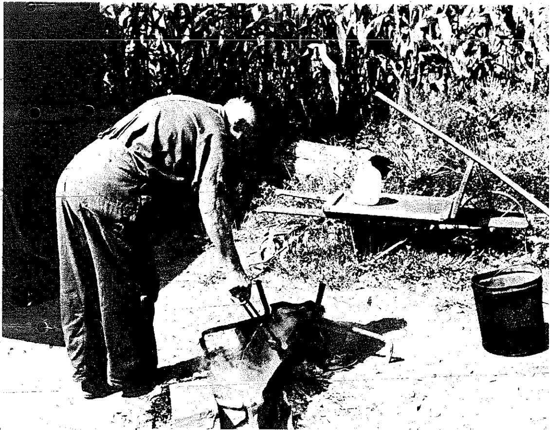
PLATE 442 Will first boils the hickory in water in a trough he designed for this purpose. Boiling the wood makes it temporarily pliable and speeds up the curing process.
