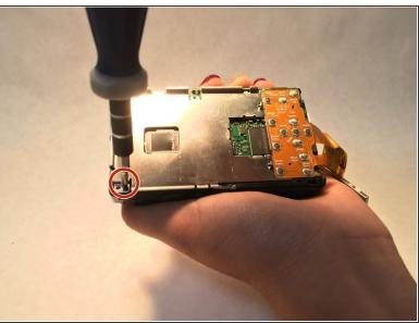
Remove the two Phillips screws. There is one at the top center and one in the bottom left corner.
