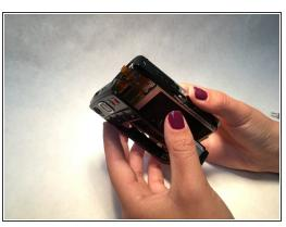
Inserting the prying tool as shown, gently separate the front and back pieces of the camera exterior.
