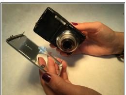
Carefully remove the front and back exterior pieces from the camera body.
