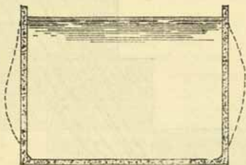
Deflection of Tank Walls.
