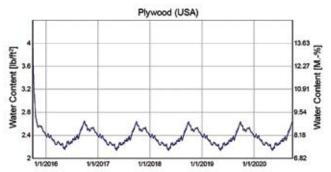
Figure 9 – Hygrothermal model graph of the plywood roof deck in the roof assembly shown in Figure 8.
