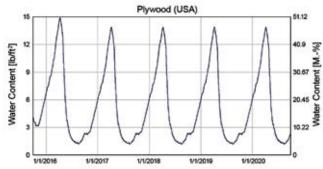
*Figure 7 – Hygrothermal model graph of the roof deck in the* roof assembly shown in Figure 1.
