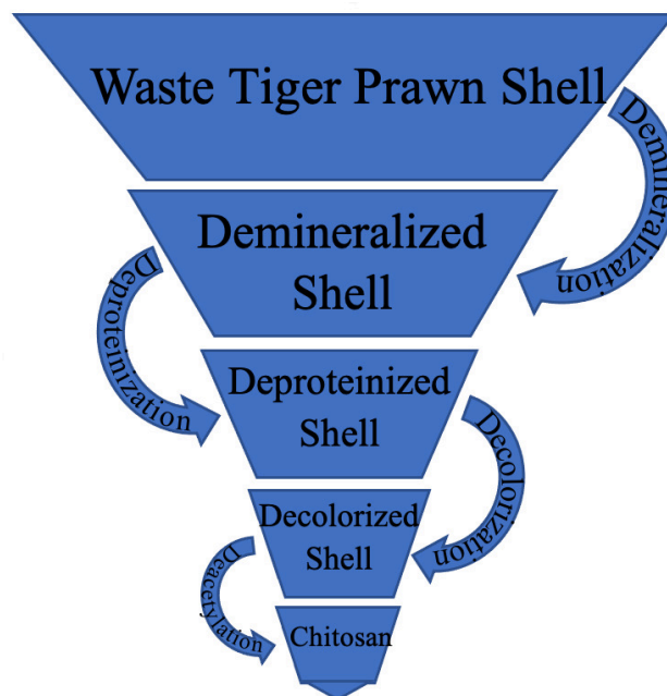
Figure 1. Chitosan Extraction from Prawn Shell Waste by Chemical Method
