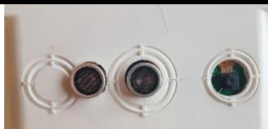
Fig. 4. PVC box with proximity sensor and camera.
