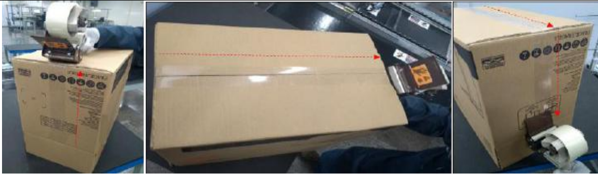
Fig. 6: Path traveled by tape passer. Source: Authors, (2018).
