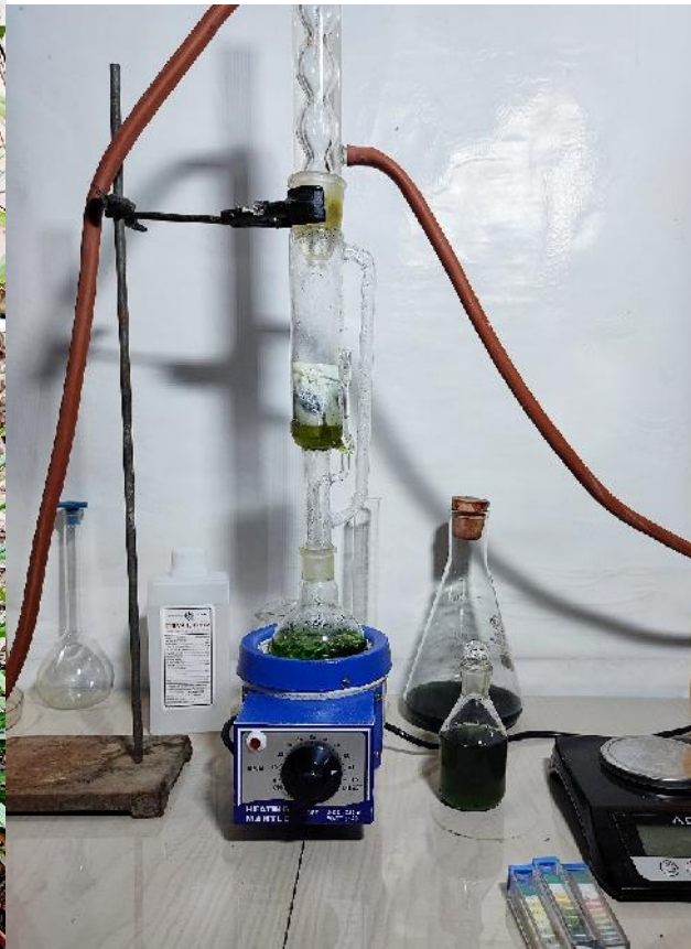
Fig.-2 Soxhlet Extraction of C. jwarancusa leaves
