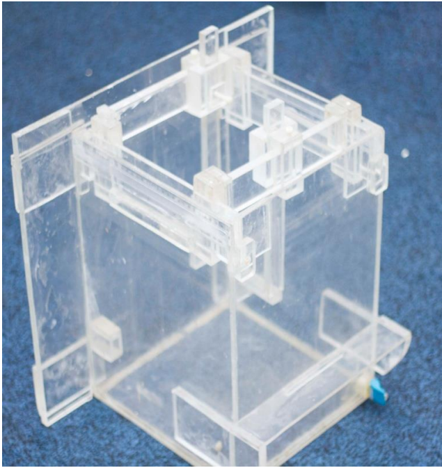
Figure 2 : Cross sectional view of the locally constructed water phantom
