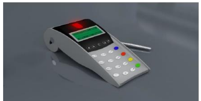
Figure 1 : The proposed POS with Embedded Fingerprint Biometric Authentication.
