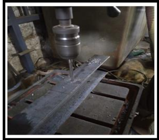
Fig. 5.4.1 Drilling of C-Chanel
